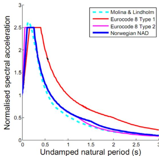
**Figure 3.** Comparison of response spectra for earthquakes in the magnitude range 5.5 to 6.0: The red curve represent Eurocode type 1 response spectrum; the blue curve represent Eurocode type 2 response spectrum; the bold magenta curve is the Norwegian NAD spectrum; and the cyan curve is uniform hazard spectrum given by Molina and Lindholm (2005). The spectra are normalized using the PGA value.
