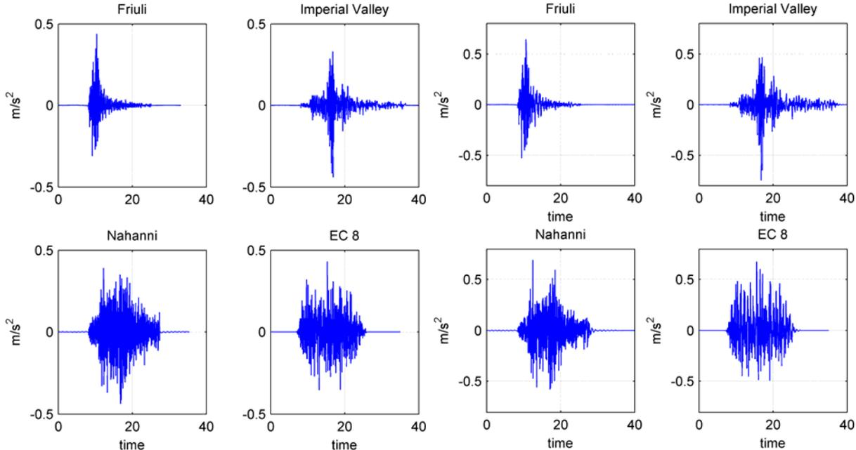
**Figure 4.** Acceleration time series of Friuli, Imperial Valley, Nahanni and EC8; bedrock (left) and clay (right)
