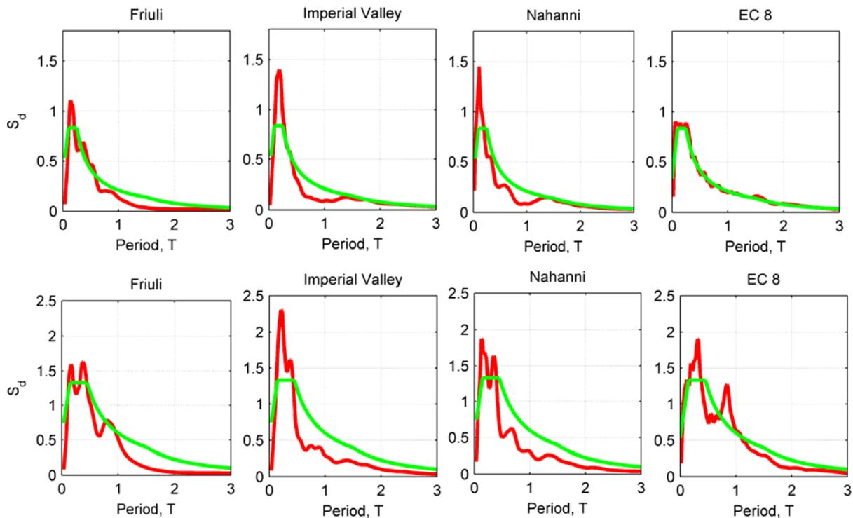
**Figure 6.** Response spectra of Friuli, Imperial Valley, Nahanni, EC 8; Bedrock (top) and Clay (bottom)
