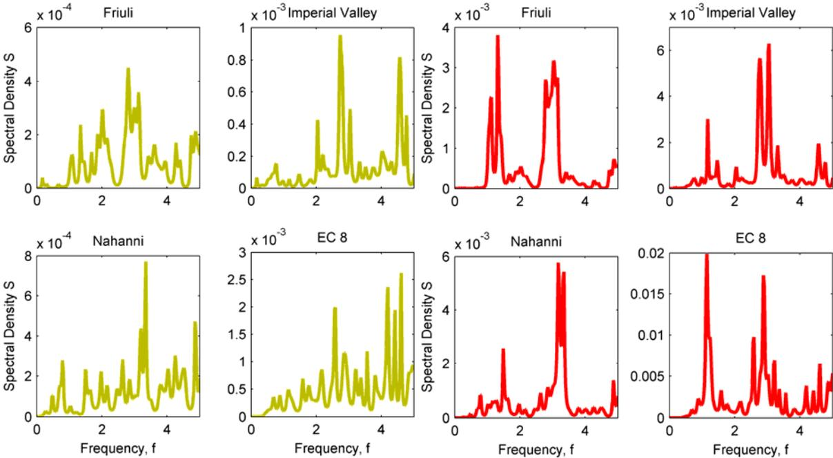
**Figure 5.** Spectral densities of acceleration time series of Friuli, Imperial Valley, Nahanni, EC 8; Bedrock (left) and Clay (right)
