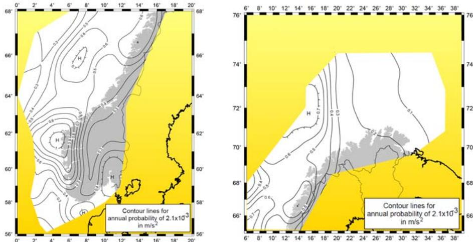
**Figure 1.** Norwegian Seismic zoning maps, contour lines for annual probability of  $2.1 \cdot 10^{-3}$ , courtesy of NORSAR
