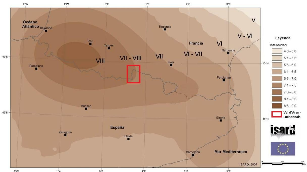
**Figure 2.1.** Seismic hazard map in terms of macroseismic intensity (return period of 475 years). (Irizarry et al., 2007).
