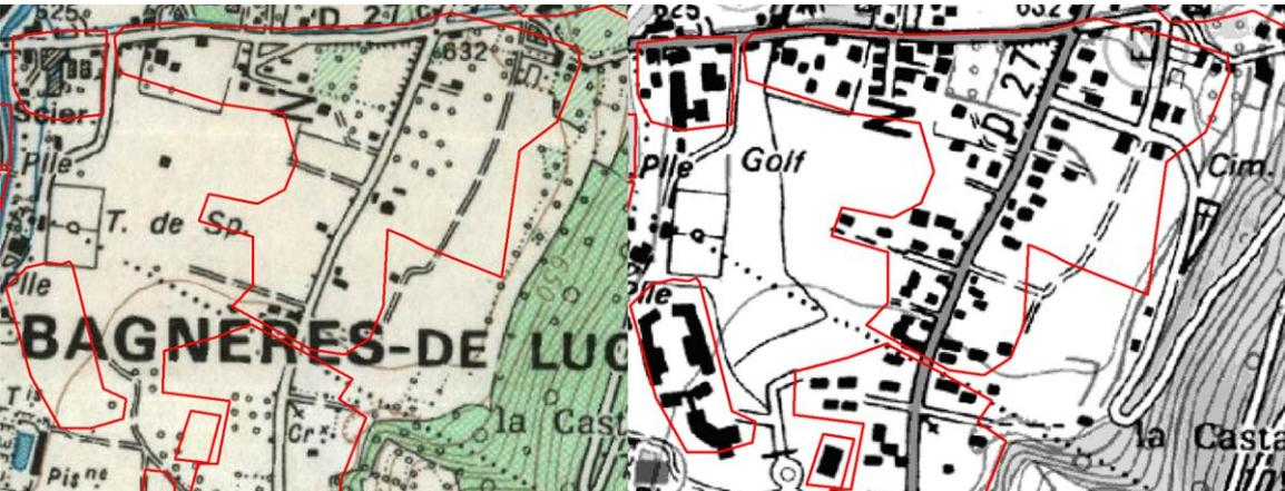
**Figure 3.3.** Example of the method to date the built zones, on the left the topographic map of 1971, on the right the newest topographic map. Almost all the buildings in the image have been built after 1971.
