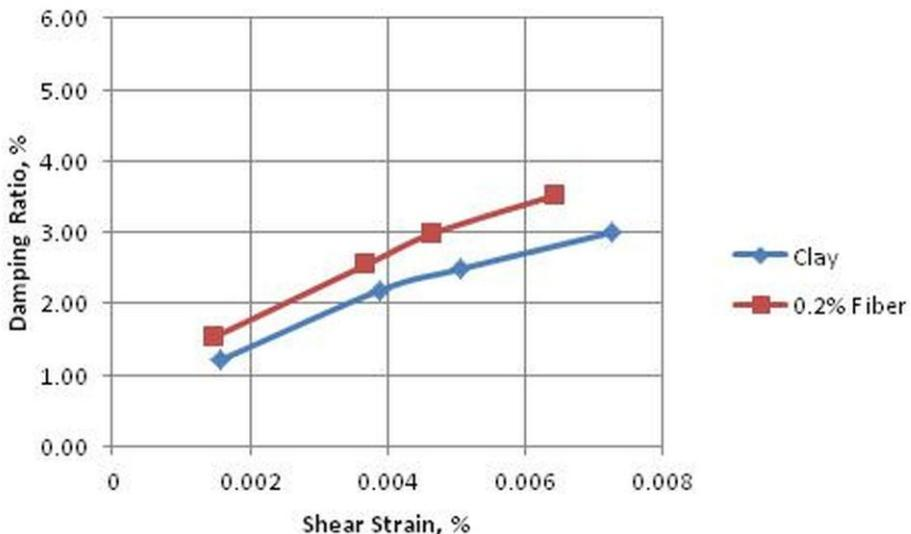
**Figure 3.** Damping ratio versus shear strain graph of clay and fiber reinforced clay
