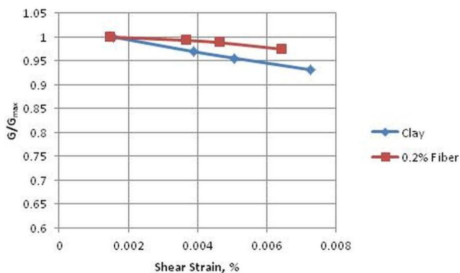
**Figure 2.** Shear modulus degradation graph of clay and fiber reinforced clay
