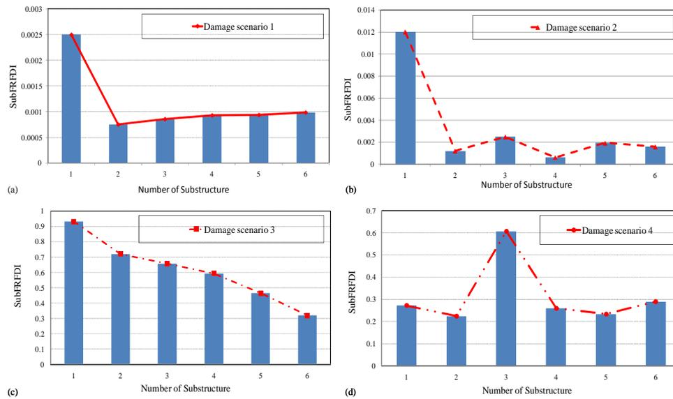
**Figure 4.** The *SubFRFDI* for damage scenarios 1–4.
