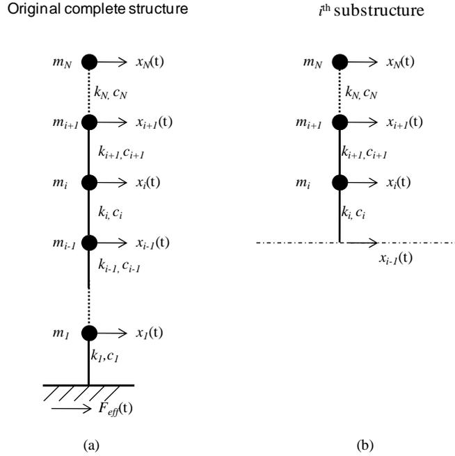
**Figure 1.** (a) Original complete structure, (b) the  $i$ <sup>th</sup> substructure.
