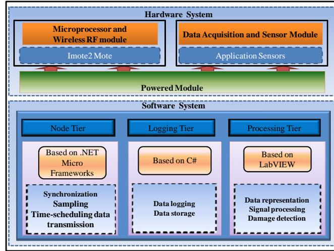
**Figure 2.** Architecture of Imote2.NET-based wireless SHM system.
