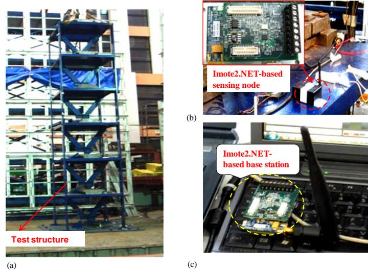
**Figure 3.** (a) A photograph of the test structure. (b) The Imote2.NET-based sensing nodes fixed on the floor. (c) The Imote2.NET-based wireless data collection base station.
