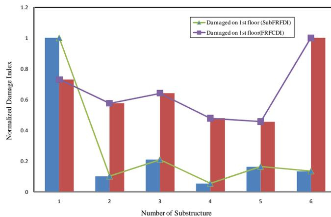
**Figure 5.** Comparison of the damage indexes obtained by the proposed *SubFRFDI* and the *FRFCDI* for damage scenario 1.
