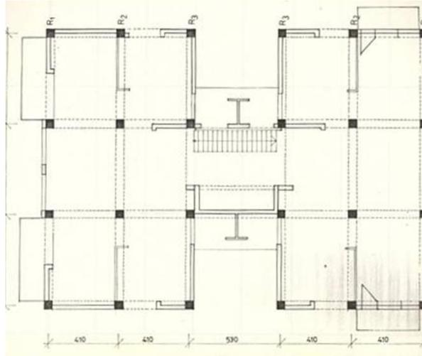
**Figure 3.1.** The floor plan of the RC building “Tower 5”
