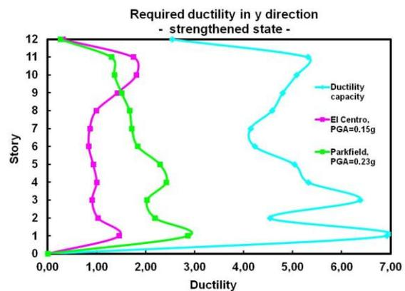
**Figure 3.4** Demand versus capacity in terms of ductilities
