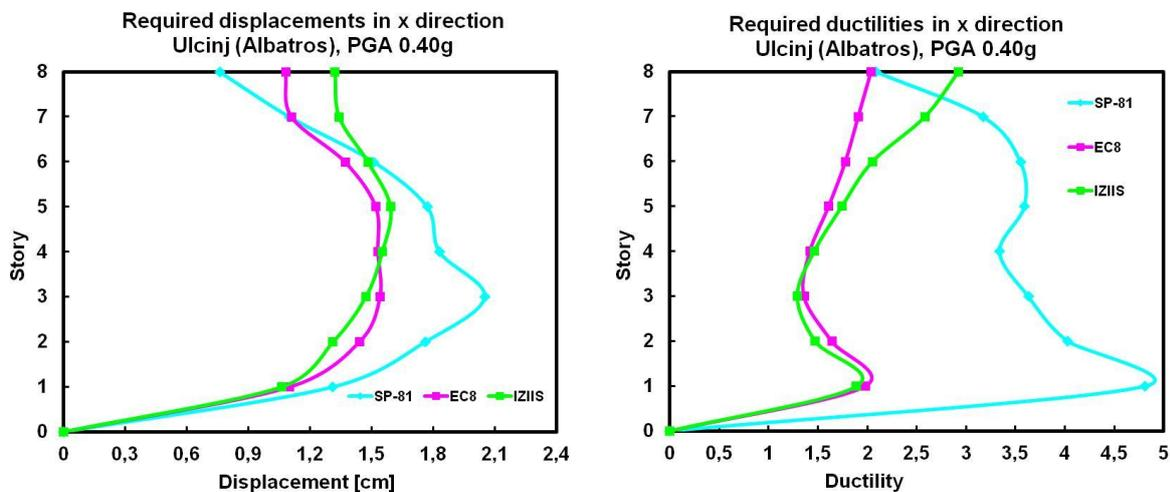
Figure 2.1. Distribution of required displacement and ductilities
