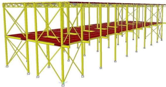
**Figure 3.8** Position of steel diagonals in the model
