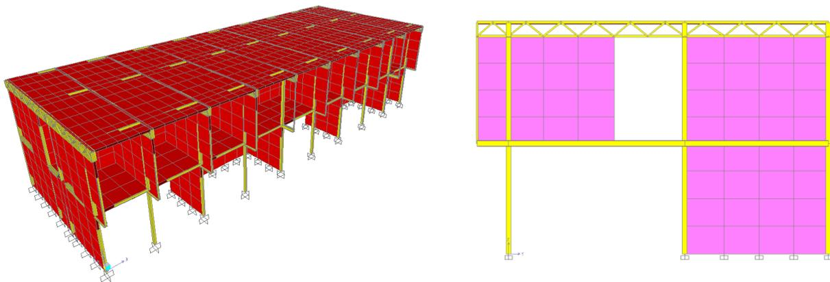
**Figure 3.6** 3D mathematical model and characteristic frame in transversal direction
