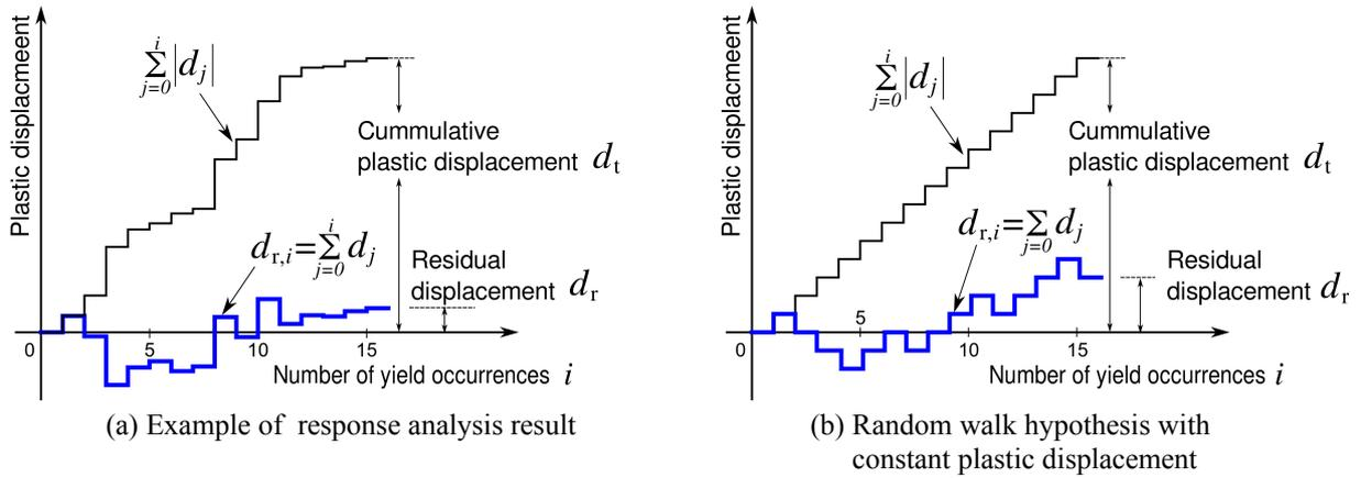
**Figure 2.** Time history of cumulative and residual plastic displacement
