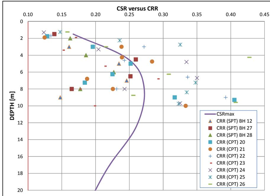
Figure 5. Liquefaction potential by SPT and CPT method (Youd et. Al., 2001)
