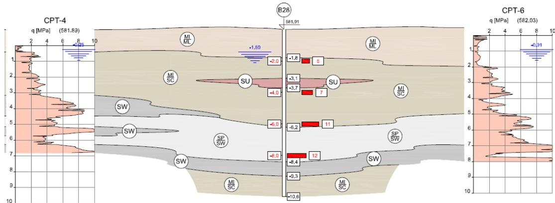
**Figure 3.** Soil profile formed on the basis of boreholes and CPT data
