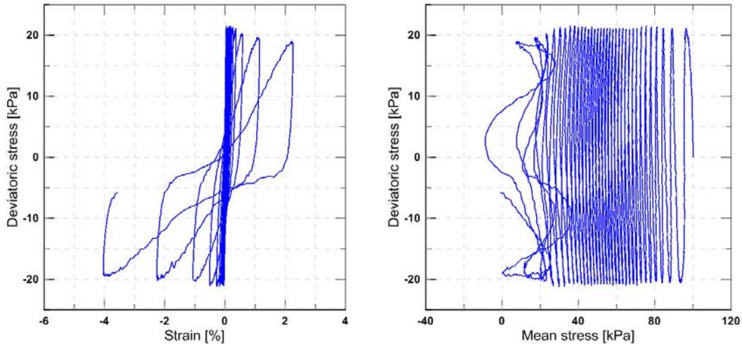
**Figure 7.** Deviatoric stress vs Strain and Mean stress vs Deviatoric stress diagrams of  $CSR=0.1$  of BH12
