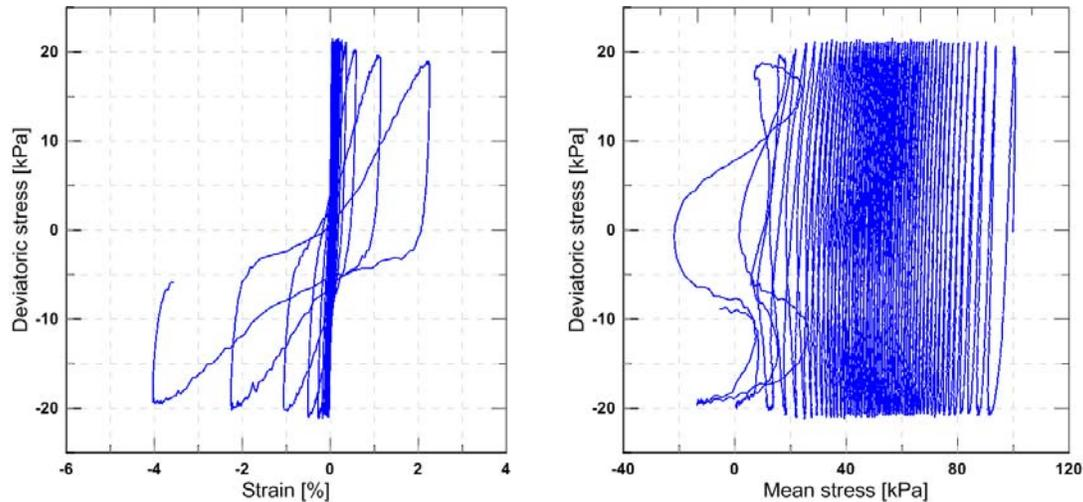
**Figure 8.** Deviatoric stress vs Strain and Meand stress vs Deviratoric stress diagrams of CSR=0.1 of BH28
