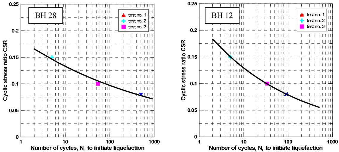
**Figure 6.** Cyclic stress ratio CSR versus number of cycles to initiate liquefaction
