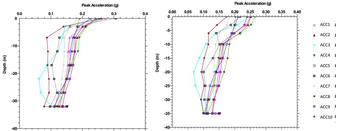
**Figure 4.** Maximum accelerations versus depth model 1(left) and model 2 (right)
