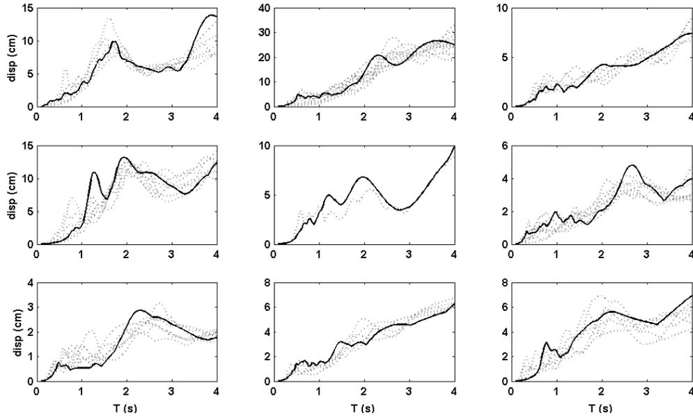
**Figure 3.** Nine of the 150 clusters employed in the IS-K method: displacement spectra of the time-series in each cluster (dashed grey) and spectrum of the randomly selected record representative of the cluster (solid black).
