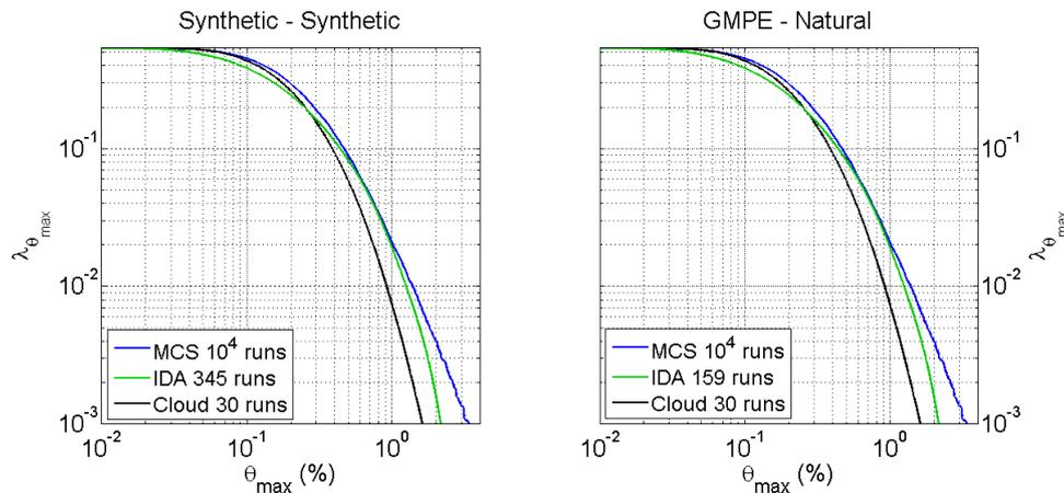
**Figure 7.** Mean annual frequency of exceedance curves of the peak inter-storey drift ratio, obtained from non-conditional and conditional approaches.
