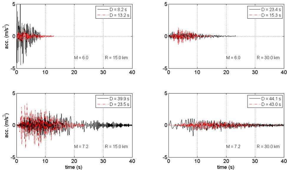
**Figure 1.** Acceleration time-series obtained from the R-ADK model for different  $(M,R)$  pairs.
