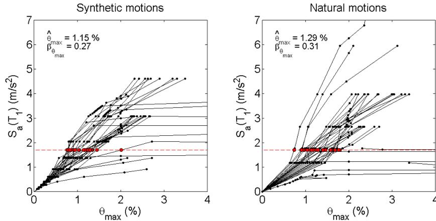
**Figure 6.** IDA curves obtained with 30 motions (synthetic on the left, natural recorded motions on the right).
