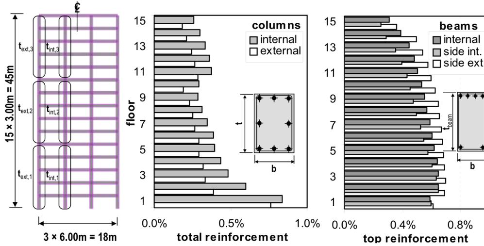
**Figure 2.** The 15-storeys RC plane frame.
