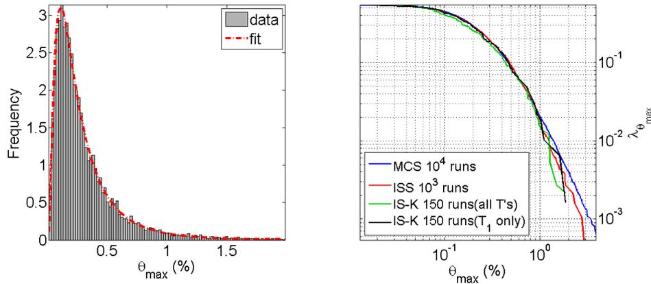
**Figure 4.** Histogram of the relative frequency of the  $\theta_{max}$  samples from the MCS (left) and MAF of exceedance of  $\theta_{max}$ , obtained from different simulation methods (right).
