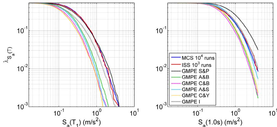
**Figure 5.** Mean annual frequency of exceedance of the spectral acceleration (hazard curve), at the first mode period  $T_1 = 2.2s$  (left) and at  $T = 1.0s$ , as obtained by PSHA with different attenuation laws (S&P: Sabetta and Pugliese 1996, A&B: Atkinson and Boore, C&B: Campbell and Bozorgnia, A&S: Abrahamson and Silva, C&Y: Chiou and Youngs, I: Idriss) and by postprocessing the spectral ordinates of the synthetic motion samples.
