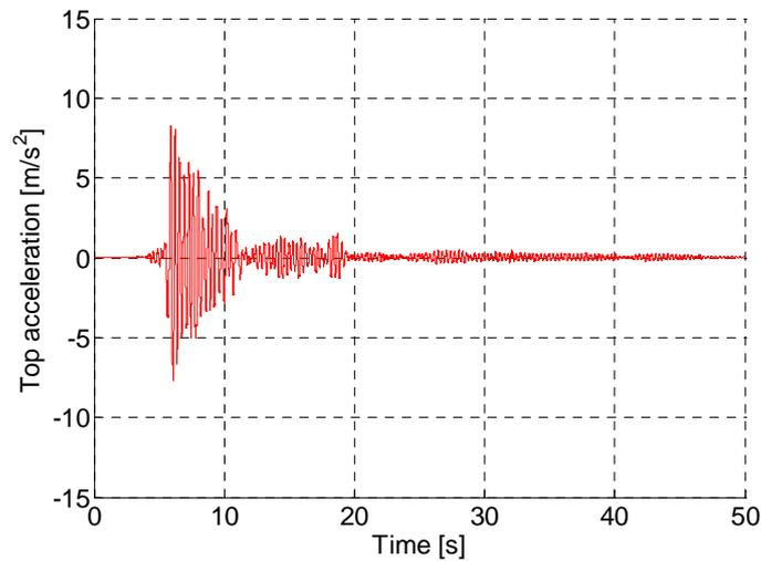
**Figure 10.** Response of the base isolated structure during the scaled Loma Prieta earthquake
