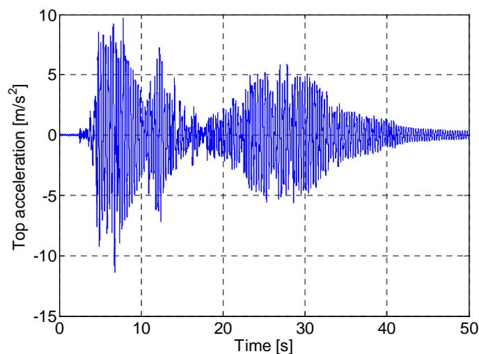
**Figure 5.** Response of the non-isolated structure during the El Centro earthquake
