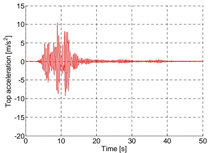
**Figure 8.** Response of the base isolated structure during the scaled San Fernando earthquake
