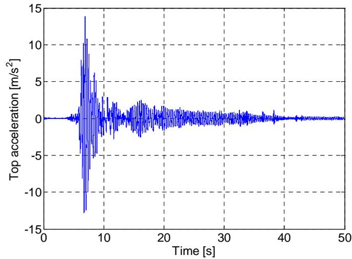
**Figure 9.** Response of the non-isolated structure during the scaled Loma Prieta earthquake
