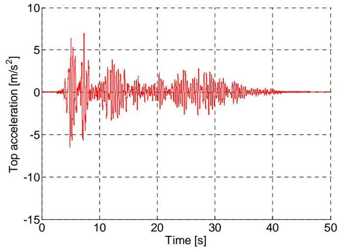
**Figure 6.** Response of the base isolated structure during the El Centro earthquake
