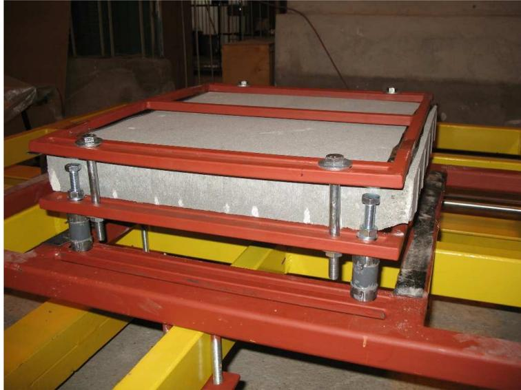
**Figure 2.** A close up view of the Elastomeric Polymer Bearings base
