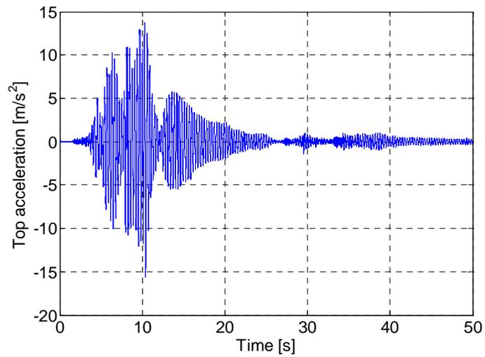
**Figure 7.** Response of the non-isolated structure during the scaled San Fernando earthquake
