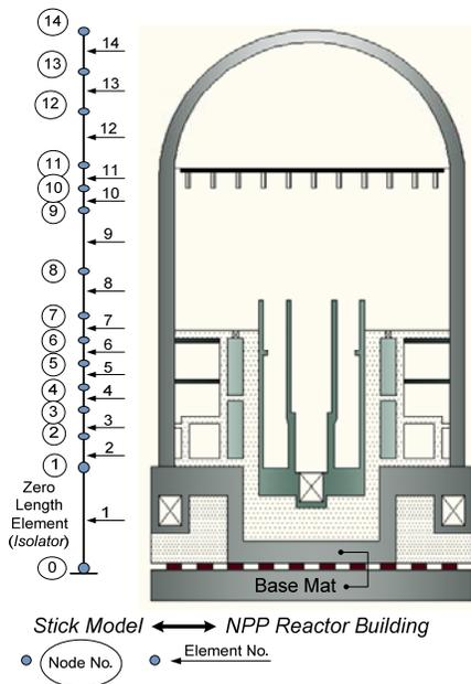
**Figure 4.** NPP reactor building and Stick Model
