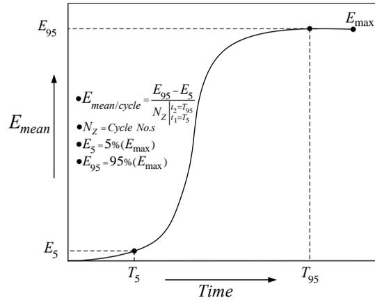
**Figure 6.** Mean hysteresis energy dissipated per cycle.
