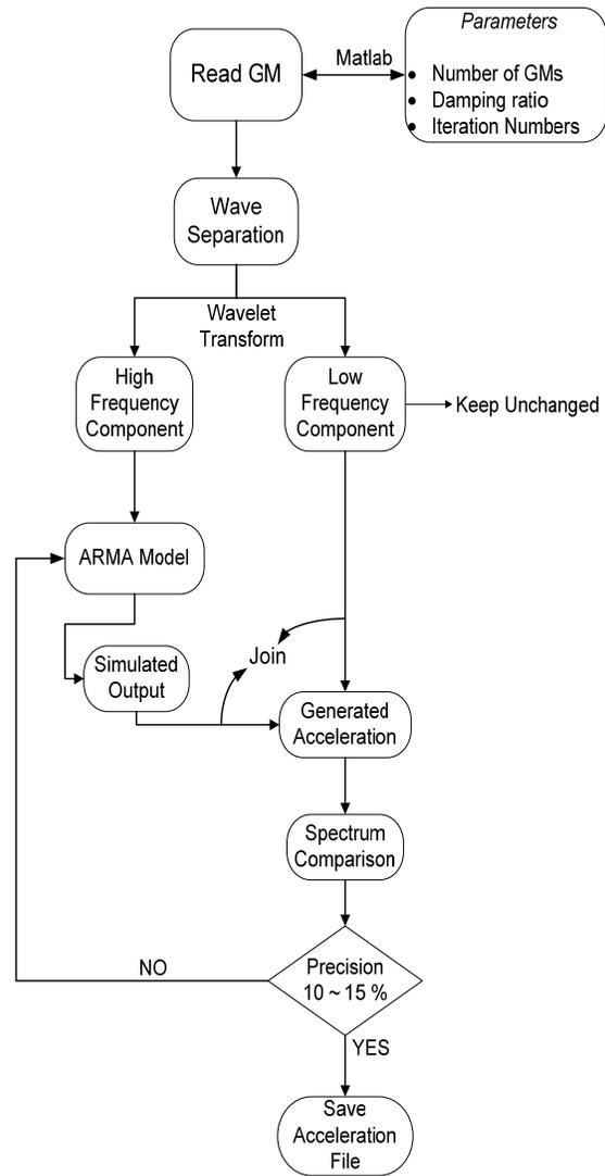
Figure 2(b). Flow Chart for simulation of long-period ground motions
