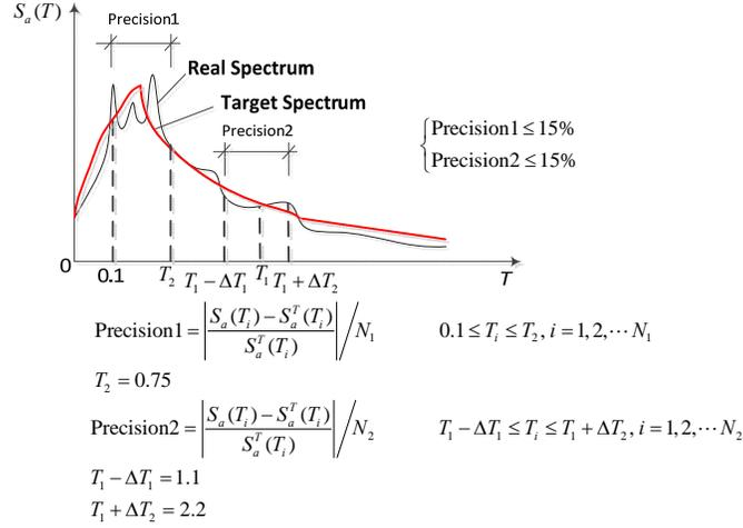
**Figure 1.** Criteria for selecting input waves for time history analyses.
