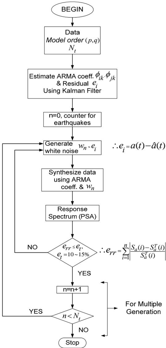
Figure 2(a). Flow Chart for ARMA simulation of short-period ground motions
