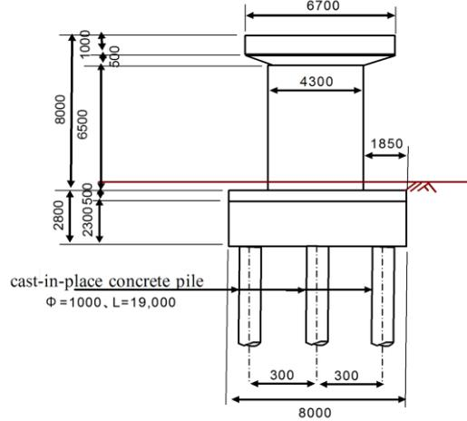
**Figure 6.** Designed RC pier ( $K_{hy} = 0.4$ )
