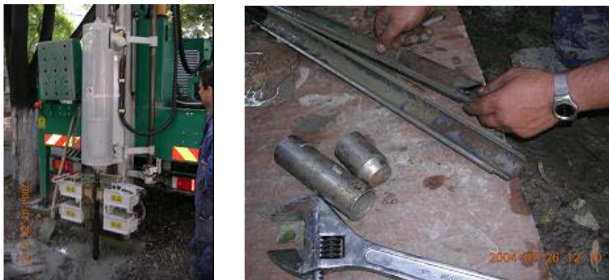
Figure 3. Standard Penetration equipment of CNRRS
