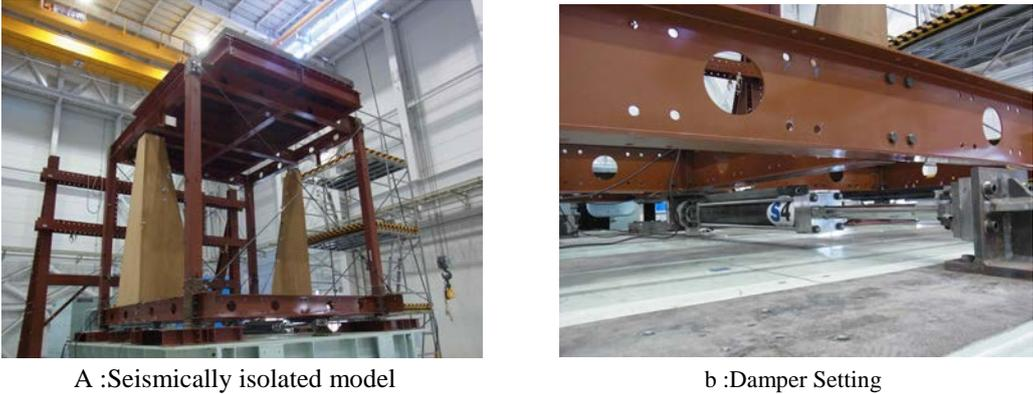
**Photograph 5.2.** Specimen and damper setting on shaking table test
