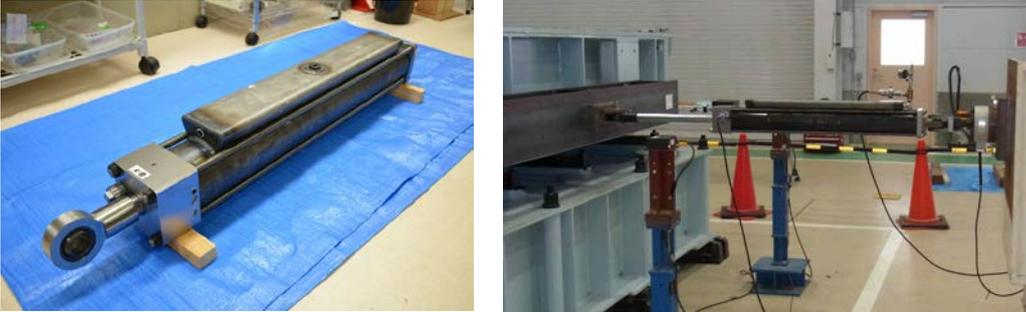
**Photograph 5.1.** Schematic view of variable damper and dynamic performance test setup
