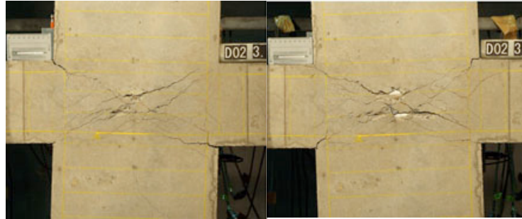
(b) Specimen D02 at story drift ratio of 3.0%
