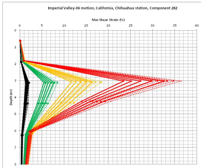
Figure 3.4. Maximum earthquake induced shear strains with AMPLE2 simulations
