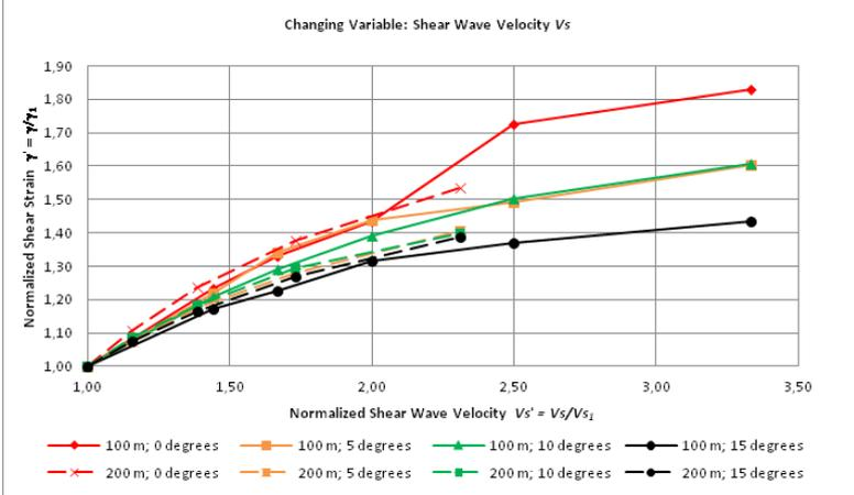
Figure 4.4. Sensitivity analysis based on shear wave velocity in half-space with AMPLE2
