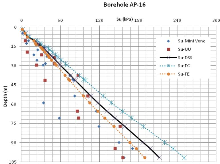
**Figure 2.1.** Undrained shear strength soil profile
