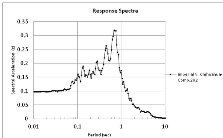
**Figure 3.3.** Response spectrum for Imperial Valley-06 motion (damping ratio  $\xi = 5\%$ )
