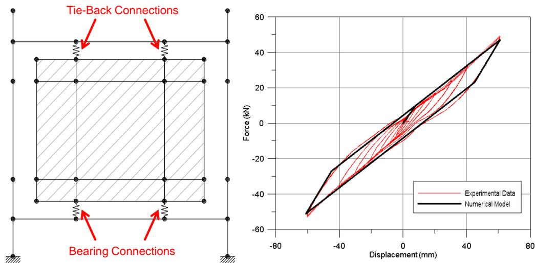
**Figure 4.1.** Cladding model in test frame model (left), numerical validation of model (right)
