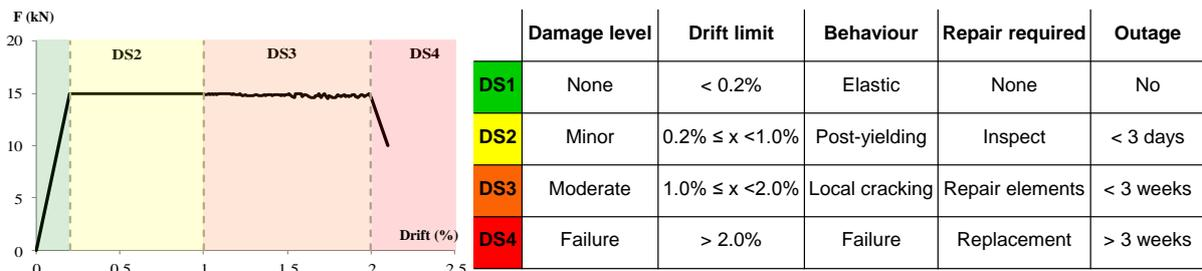
**Figure 3.4.** Damage states definition
