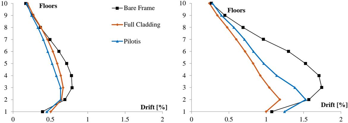
**Figure 5.4.** Mean interstorey drift of different building configurations for DBE (left) and MCE (right)
