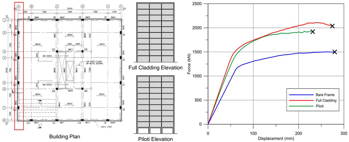
**Figure 5.1.** Pushover analysis response of cladding systems compared to bare frame
