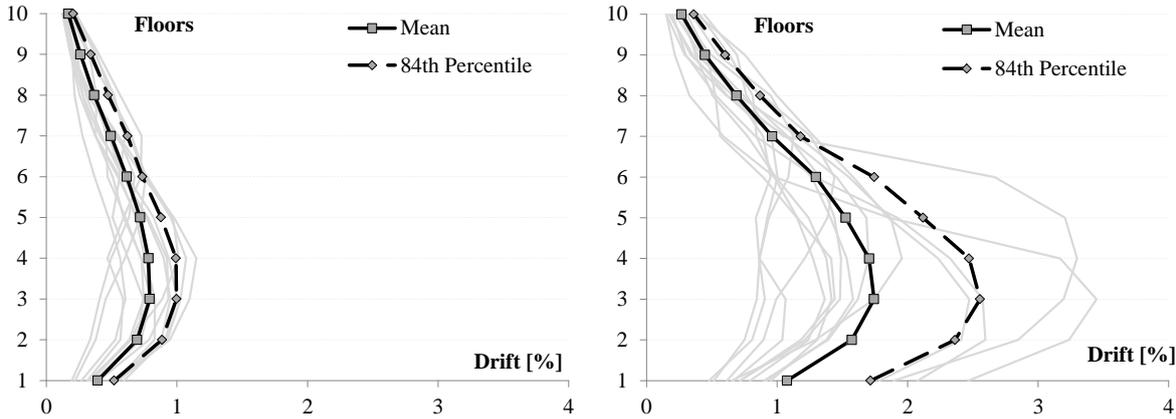
**Figure 5.3.** Interstorey drift of the bare frame building for DBE (left) and MCE (right)
