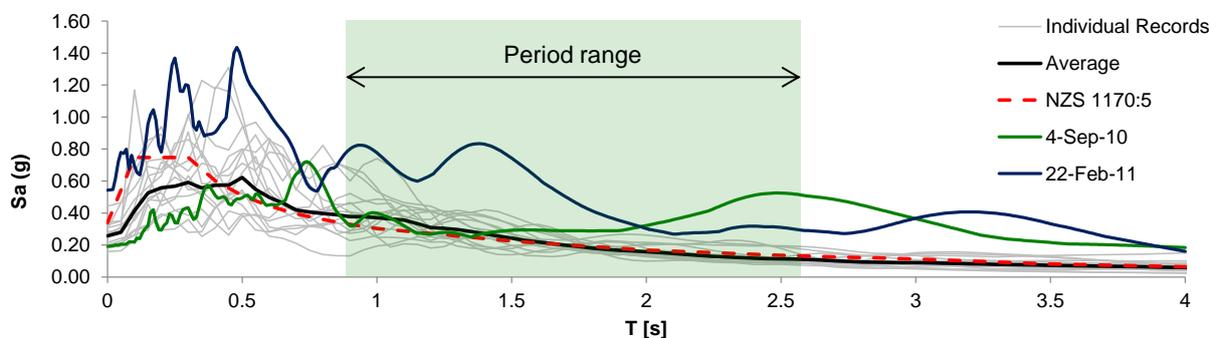
**Figure 5.2.** Scaled fifteen accelerograms and average compared with NZS 1170.5 design spectrum and Christchurch earthquake records
