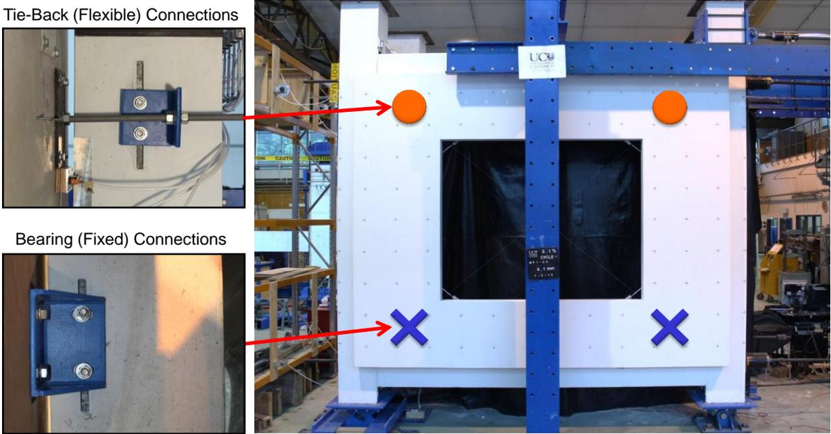
Figure 3.2. Experimental test frame with cladding showing connection assemblies
