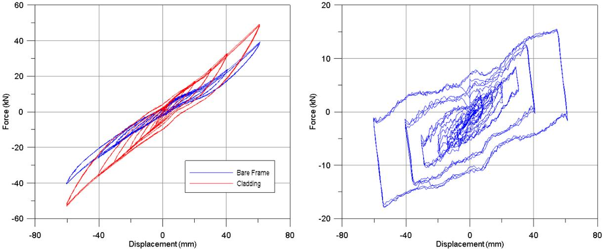
Figure 3.3. Comparison of bare frame and clad frame (left), contribution to frame by cladding (right)
