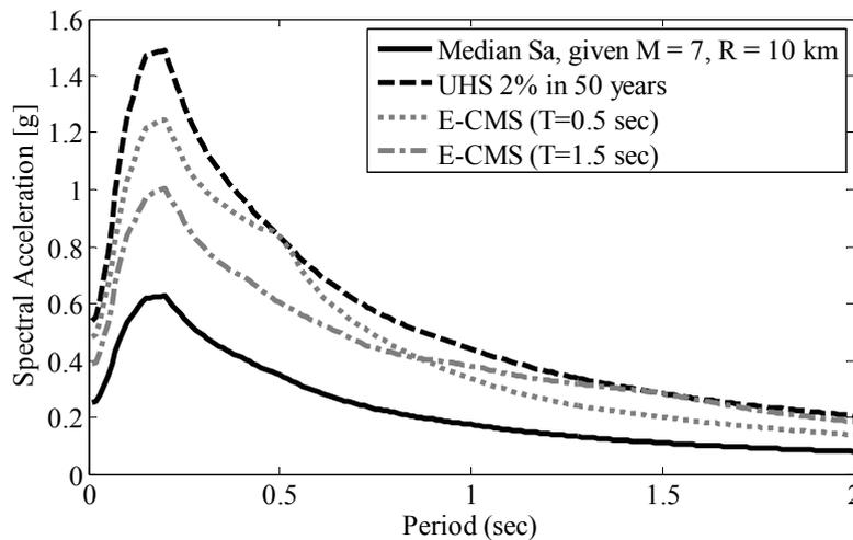
**Figure 6.** Eta-based conditional mean spectra in different periods for an equal probability of exceedance 2% in 50 years. ( $T^*=0.5$  sec &  $T^*=1.5$  sec).
