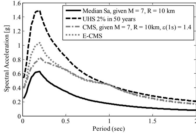
**Figure 4.** UHS, Epsilon-based and Eta-based conditional mean spectrum for an ideal site, given M=7, R=10 km, ε=1.4.
