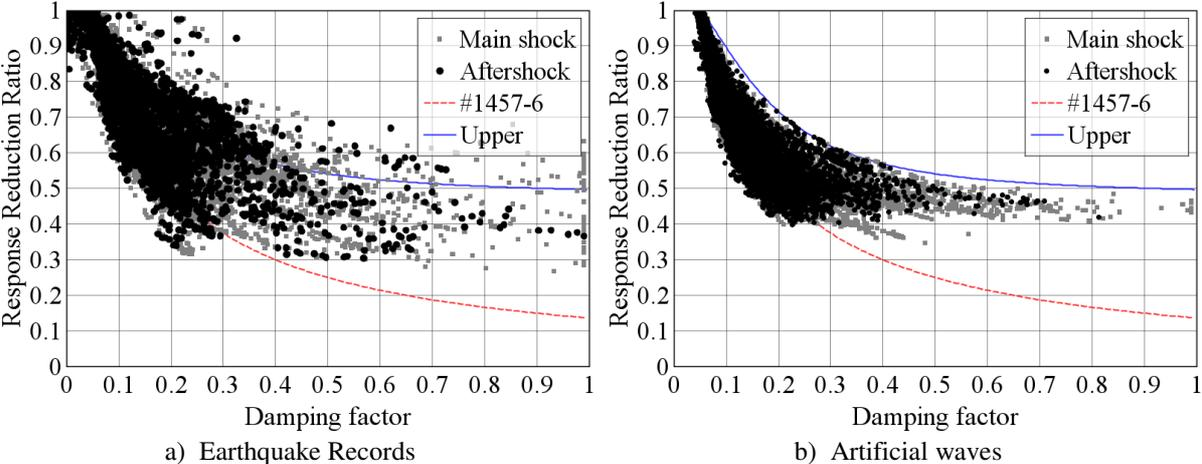
**Figure 4.2.** Relationship between response reduction ratio and damping factor for Takeda Model
