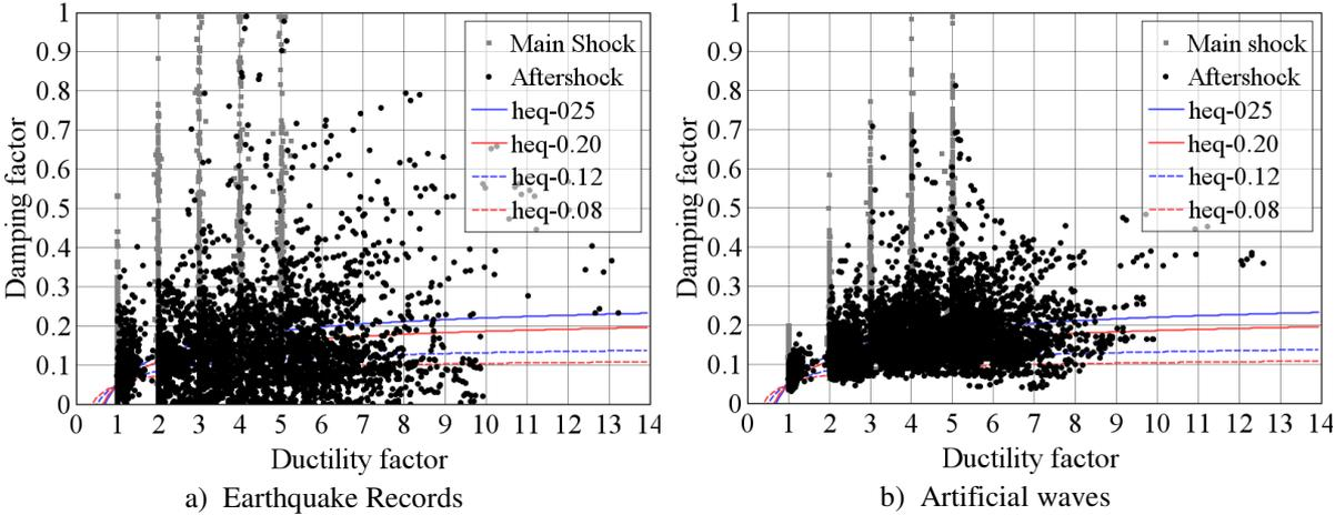
**Figure 4.1.** Relationship between damping factor and ductility factor for Takeda Model
