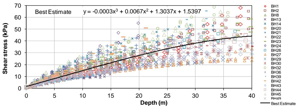
**Figure 4.** Maximum shear stress against depth for all boreholes for ‘2% chance of being exceeded in the next 50 years’ near-field ground motion
