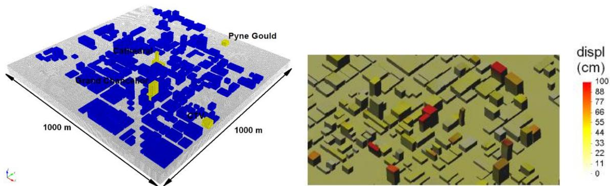
**Figure 2.1.** Left: 3D-model of the soil and the buildings in Christchurch CBD, Guidotti (2012)
