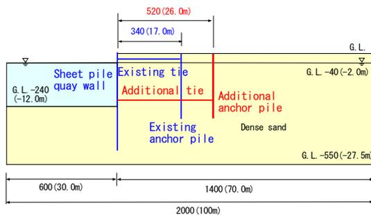
**Figure 2.1** Model P1 (Horizontal reinforcement tie)
