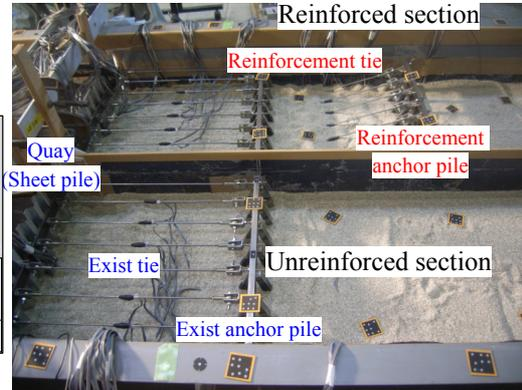
**Figure 2.4** Photo of the model during preparation
