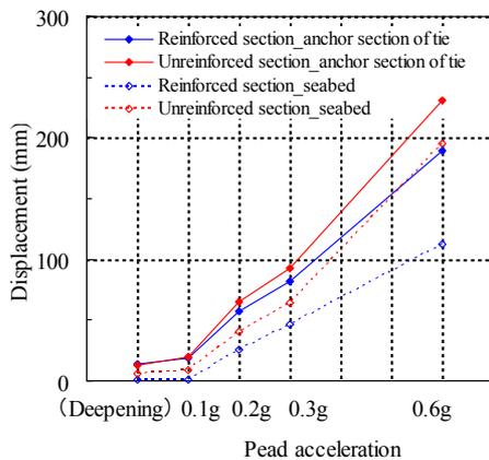
**Figure 2.10** Comparison of the maximum horizontal displacement of quay-wall (Sea ward +)
