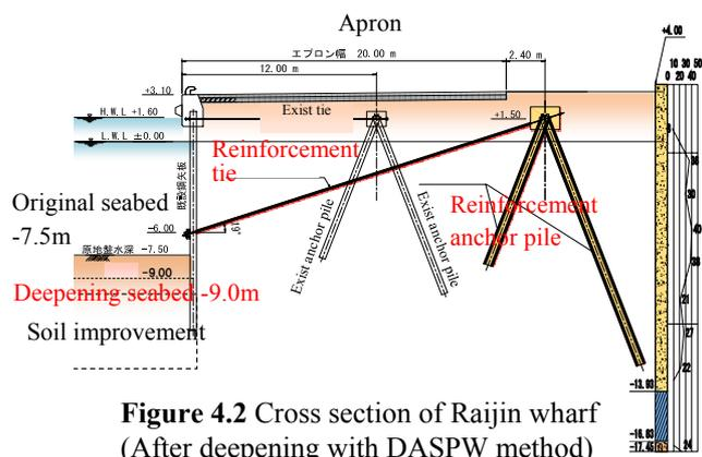
Figure 4.2 Cross section of Raijin wharf (After deepening with DASPW method)
