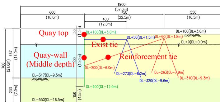
**Figure 3.1** Simulation model and locations of major outputs for comparison
