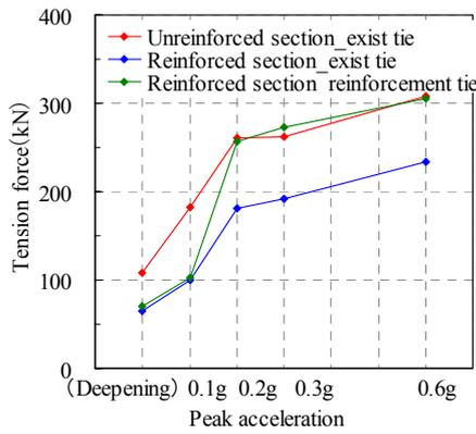
**Figure 2.9** Comparison of the maximum axial force of ties (Tension)
