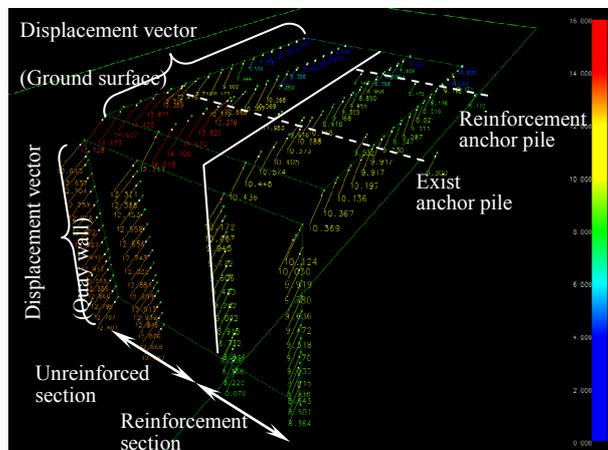
**Figure 2.11** Deformation of quay-walls and back yards determined by image analysis (Sea ward: left)
