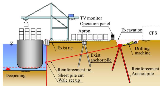
**Figure 1.1** Conceptual drawing of the dual anchored sheet pile wall method (constructed by UGETS)
