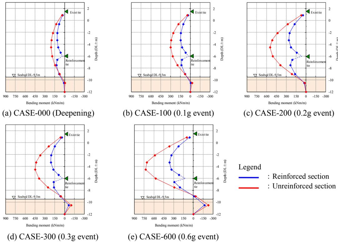
**Figure 2.8** Comparison of the maximum bending moment distributions throughout the quay-wall
