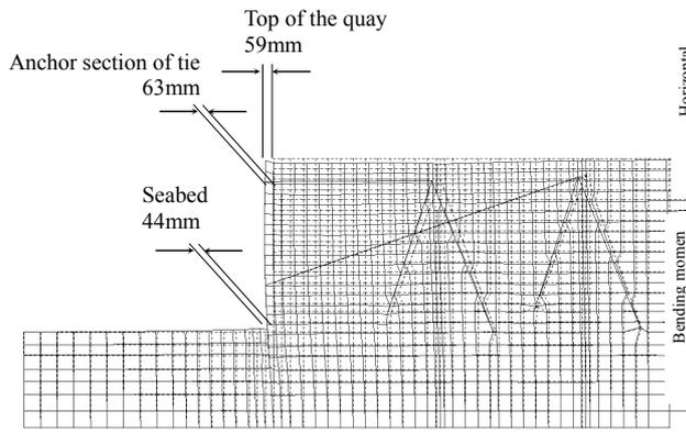
**Figure 3.3** Deformation of whole model (Maximum deformation, CASE-A200)
