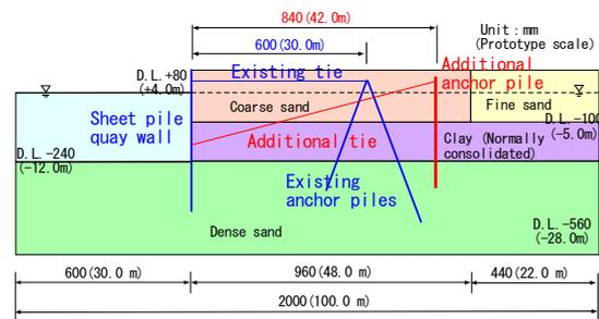
**Figure 2.2** Model P2 (Slanting reinforcement tie)
