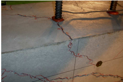
Figure 10. Pictures of post-installed anchors in ultimate state
