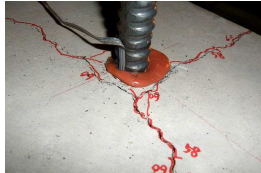
Figure 10. Pictures of post-installed anchors in ultimate state
