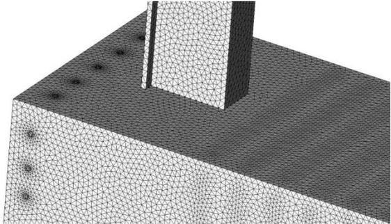
Figure 4.3. Analytical model of reinforcements and girder. Figure 4.4. Analytical model of concrete and girder
