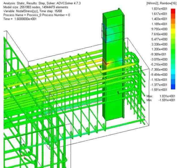
Figure 4.8. Stress distribution of rebars and girder without failure analysis.
