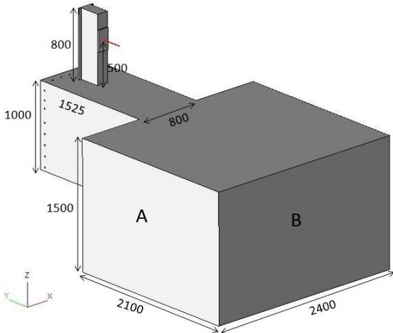
Figure 4.1. Tunnel junction member model (unit: mm).
