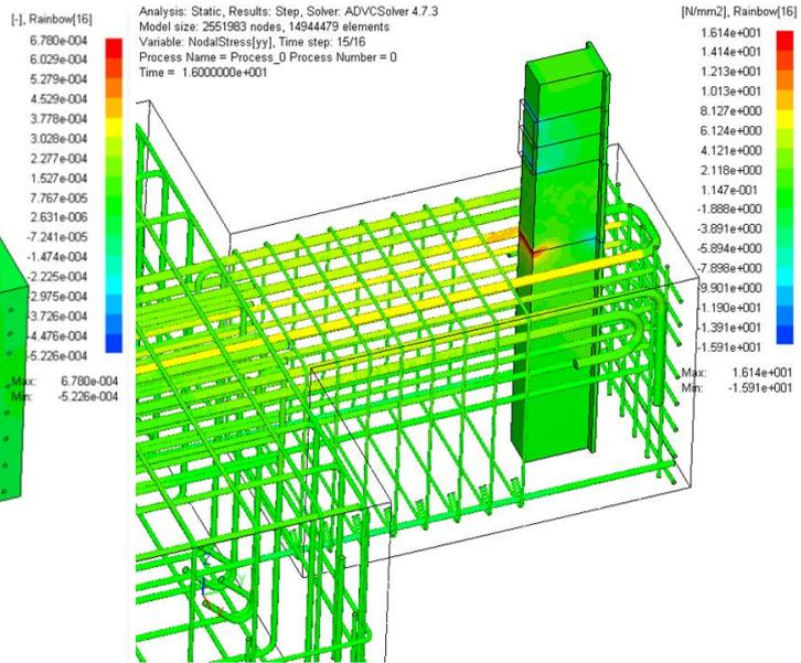
Figure 4.6. Stress distribution for rebars and girder with failure analysis.
