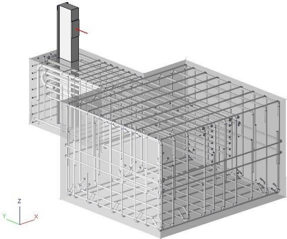
Figure 4.2. Model of reinforcements and girder
