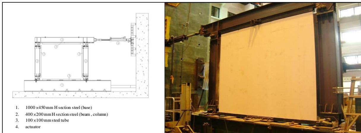
**Figure 3.** Details of the test frame
