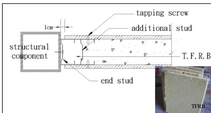
**Figure 5.** Details of the W6 specimen
