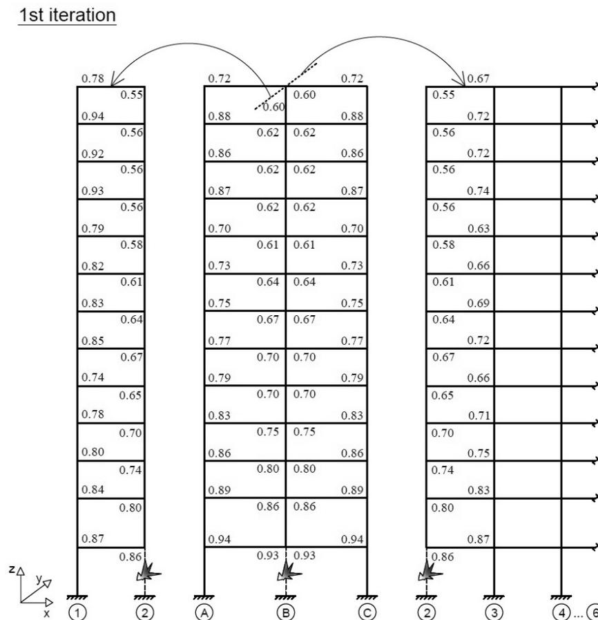
Figure 4.3. DCR values for flexure in the damage case C<sub>4</sub> - Bucharest model designed for high ductility class
