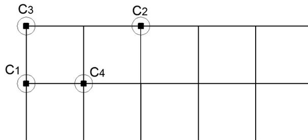
**Figure 3.1.** Damage cases according to the GSA (2003) Guidelines
