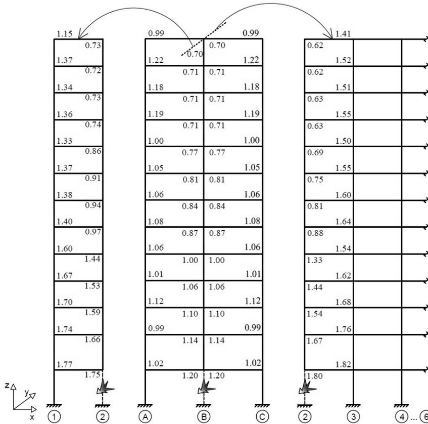
Figure 4.1. DCR values for flexure in the damage case  $C_4$  - Cluj model designed for medium ductility class
