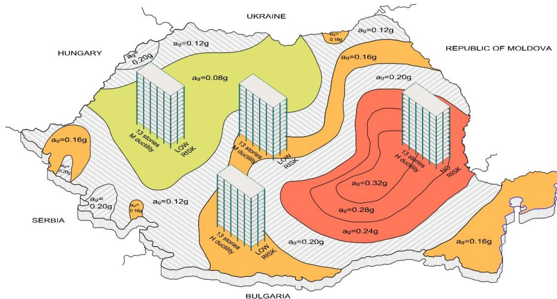
**Figure 5.1.** Progressive collapse safety map for mid-rise structures in Romania
