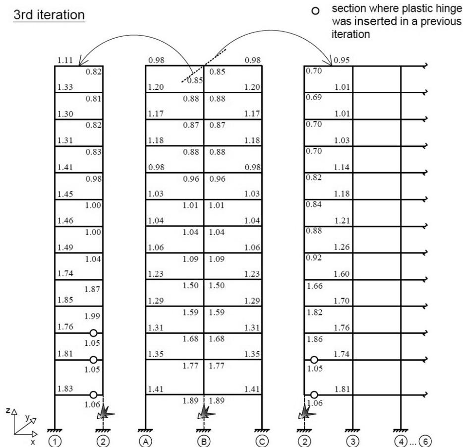
**Figure 4.2.** DCR values for flexure in the damage case C<sub>4</sub> - Sibiu model designed for medium ductility class
