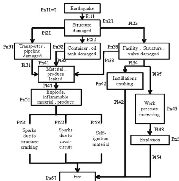
Figure 2.2. Earthquake & fire links in disaster chain of petrochemical industry system
