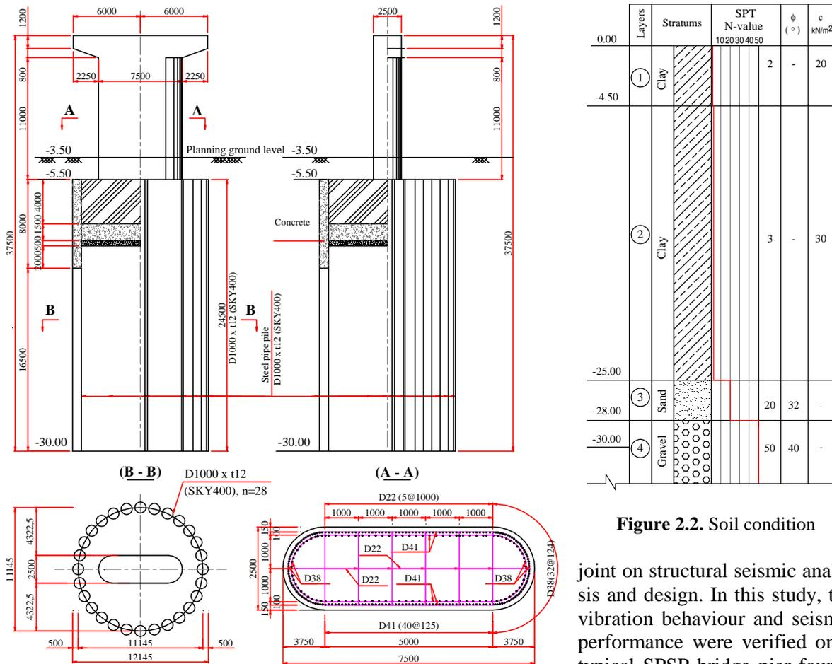
Figure 2.1. Prototype bridge pier-SPSP foundation
