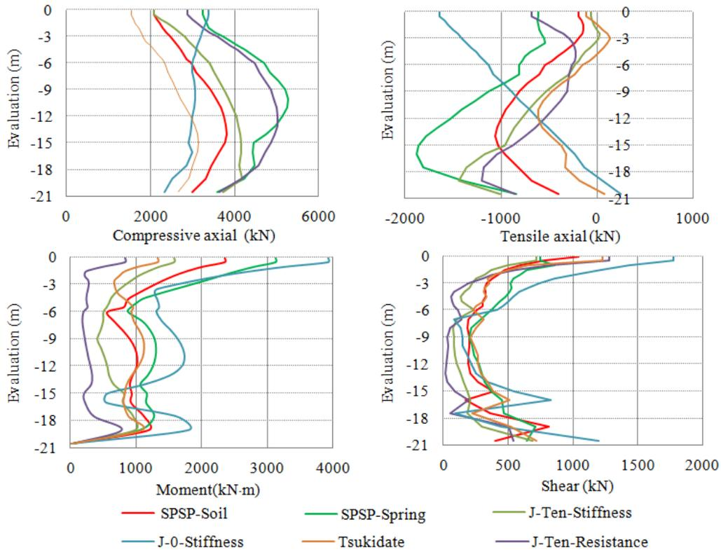
**Figure 8.2.** Sectional forces distribution of the pile
