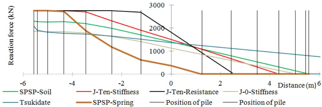
**Figure 8.3.** Vertical reaction forces at the ends of the pile
