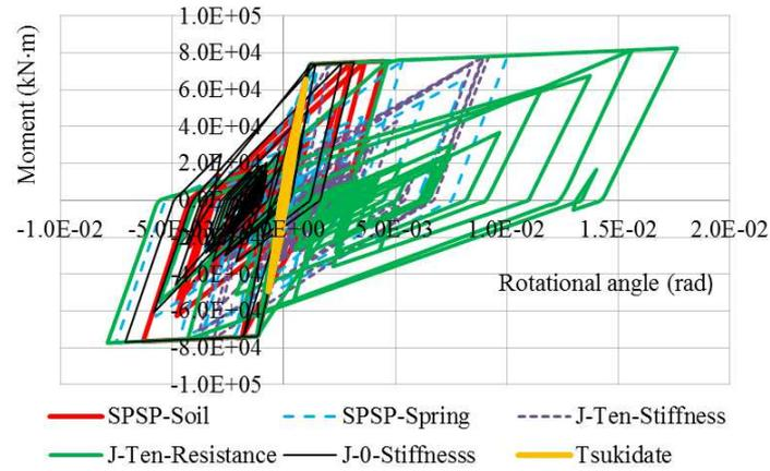
**Figure 8.1.** Hysteresis loop of bending moment against rotational angle of plastic hinge
