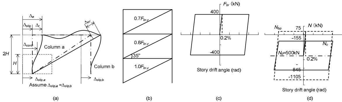
**Figure 3.** (a) Frame deformation; (b) prototype frame;
