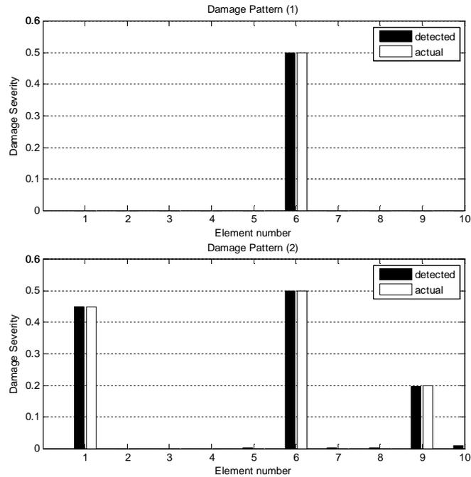
**Figure 4.2.** The obtained results for two damage patterns of the simply supported beam
