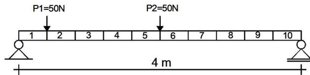
**Figure 4.1.** The simply supported beam with the finite element model
