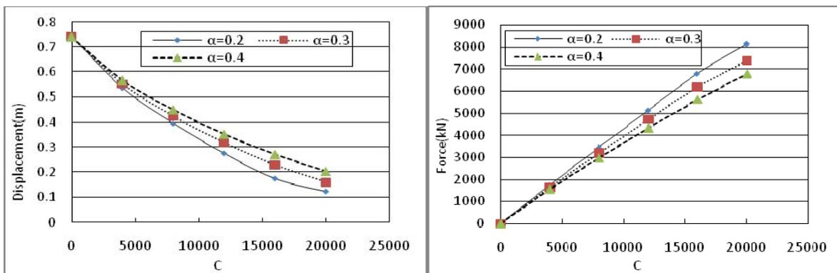
Fig.5.1 Displacement of the damper
