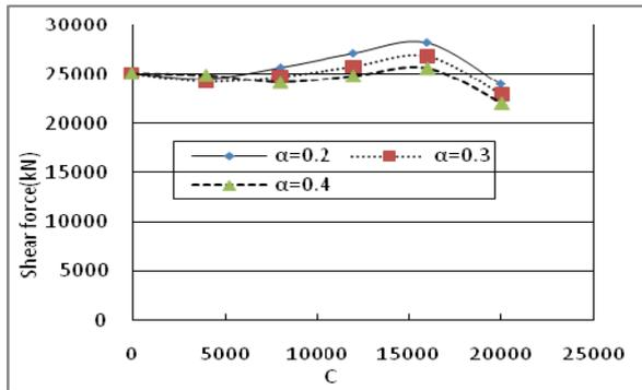
**Fig.5.5** Shear force at the base of the pylon
