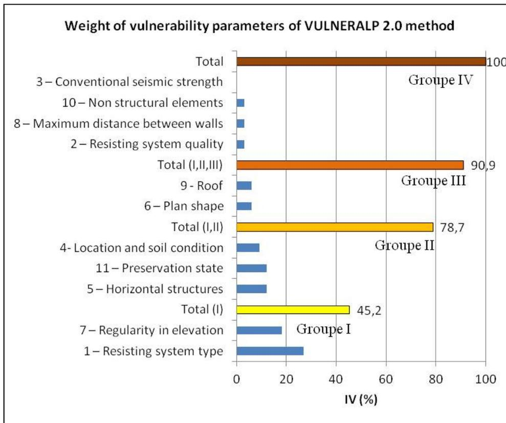
Figure 2: Relative weights of the 11 vulnerability parameters for VULNERALP2.0 method
