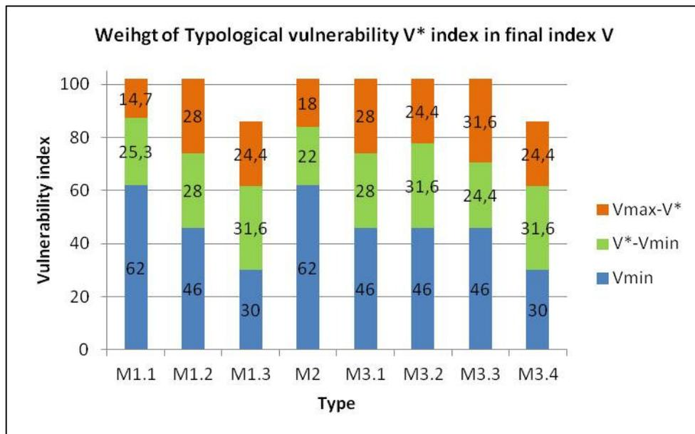
Figure 3: Range of variation of the vulnerability index V\* (from Vmin to Vmax) for the main RISK-EU masonry typologies
