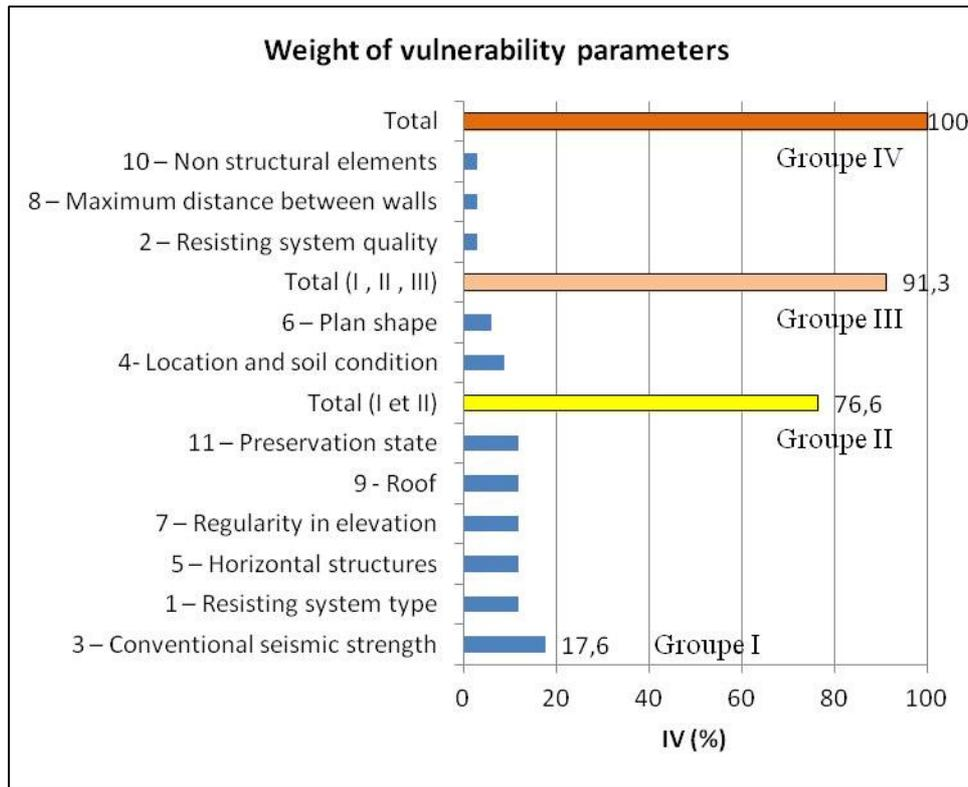
Figure 1: Relative weights of the 11 vulnerability parameters - GNDT Method
