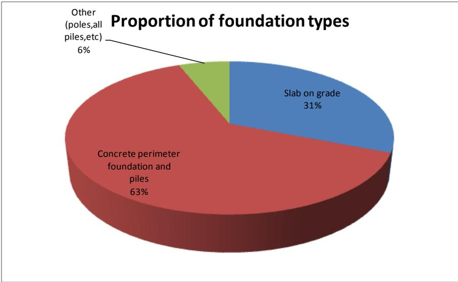
**Figure 2.** Proportions of foundation types in surveyed structures
