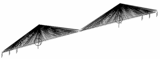
**Figure 3.7.** Locations of viscous dampers
