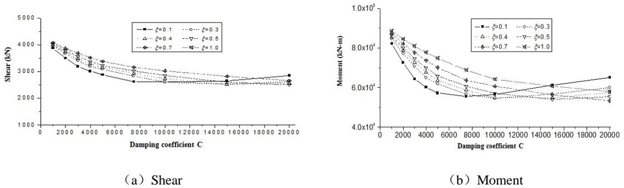
**Fig.3.13.** Influence of damping coefficient  $C$  and velocity exponent  $\zeta$  on internal forces at the middle tower base
