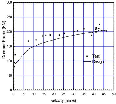
**Figure 3.5.** Damper force versus velocity for all cyclic constant-velocity tests
