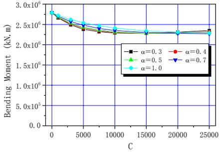
Figure 3.11. Bending moment at the base of tower
