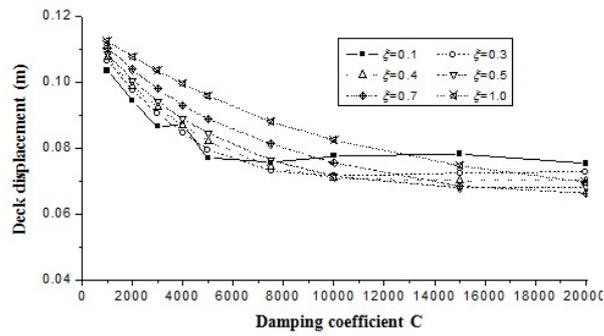
**Fig.3.12.** Influence of damping coefficient  $C$  and velocity exponent  $\zeta$  on deck displacement on the north side
