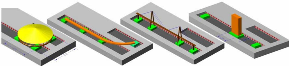
**Fig. 4.1** Working modes of the Tongji shake table array
