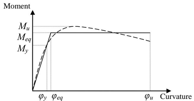
**Fig 2.3.** Moment-Curvature curve
