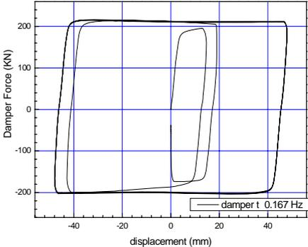
**Figure 3.4.** Typical damper force versus displacement plot for a cyclic constant-velocity test
