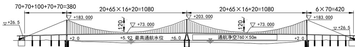
Figure 2.1. The overall layout of the Taizhou Bridge
