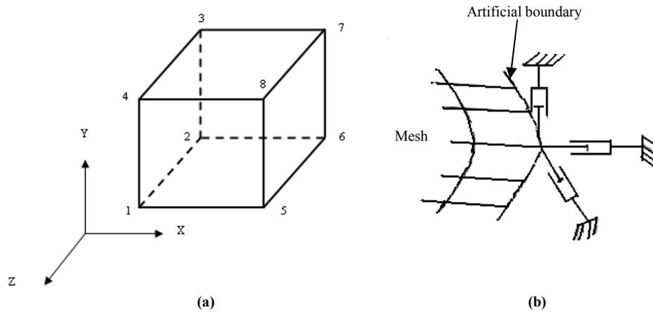
**Figure 2.** (a) Eight-node Hexahedral element (b) Viscous damper on the boundary
