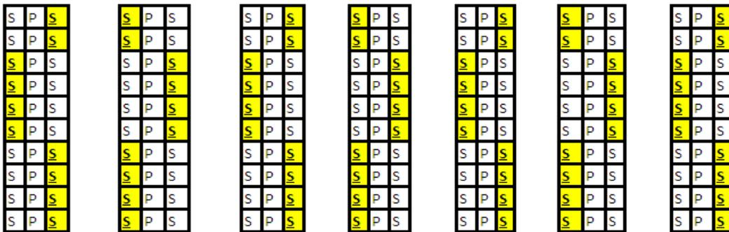
**Figure 12.** Representation of Pile and adjacent soil elements for plastic soil case of medium clay for one length of pile (with Interface Element)
