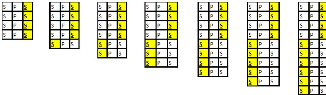
**Figure 9.** Representation of Pile and adjacent soil elements for plastic soil case of very soft clay for varying lengths of pile (with Interface Element)
