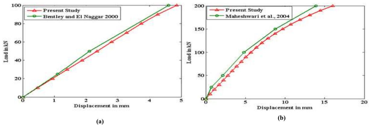
Figure 6. Response of single socketed pile for plastic soil case (a) Without Interface Element (b) With Interface Element.
