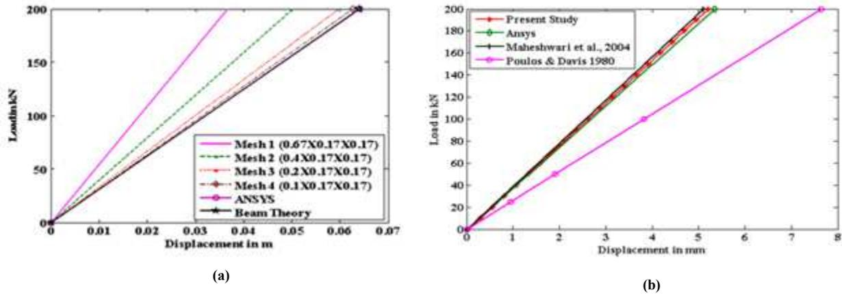
Figure 5. Response of pile (a) As Cantilever (b) Embedded in soil.
