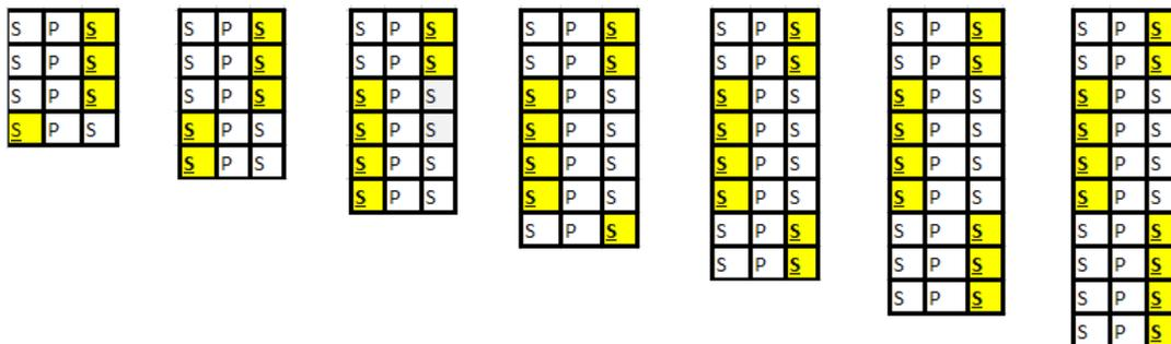
**Figure 10.** Representation of Pile and adjacent soil elements for plastic soil case of medium clay for varying lengths of pile (with Interface Element)
