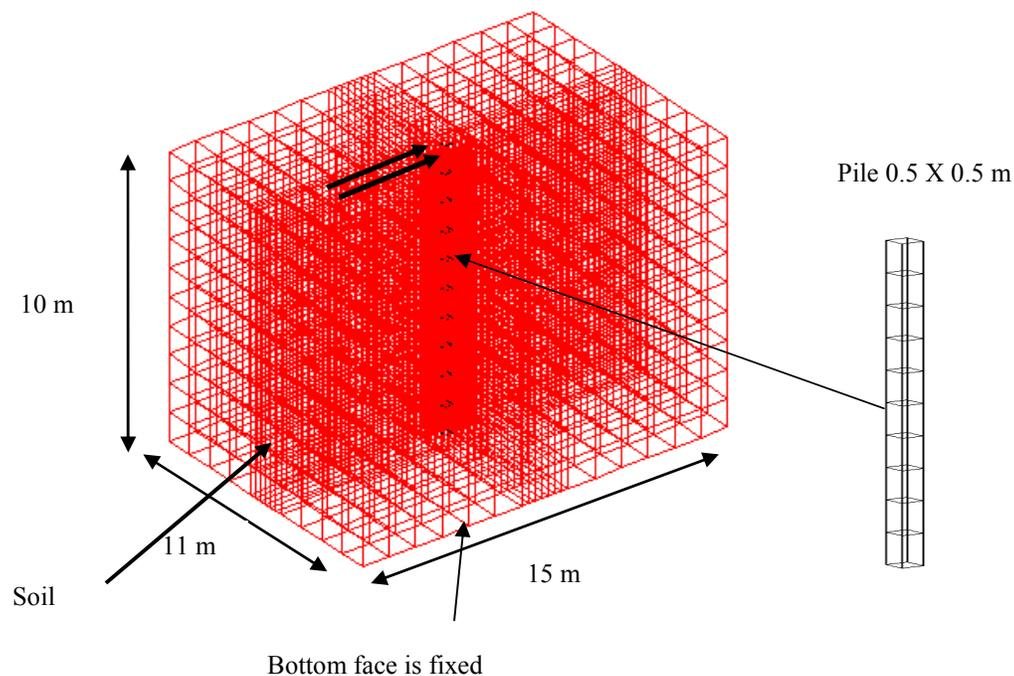
**Figure 1.** 3D pile soil system considered for the study
