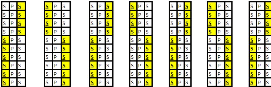
**Figure 11.** Representation of Pile and adjacent soil elements for plastic soil case of very soft clay for one length of pile (with Interface Element)
