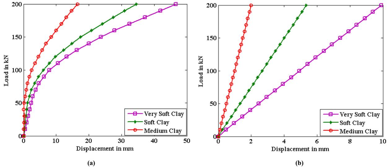
**Figure 8.** Response of single socketed pile for various soils in plastic state
