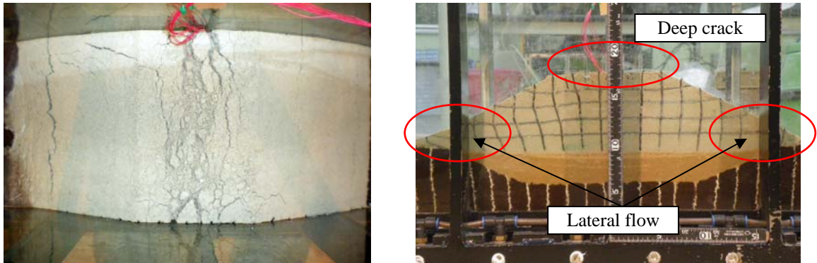
Photo 3. Case 3 without countermeasures (input acceleration: 275 \text{ m/s}^2 ) (Left: situation at the top of the embankment; right: situation as seen from the side)
