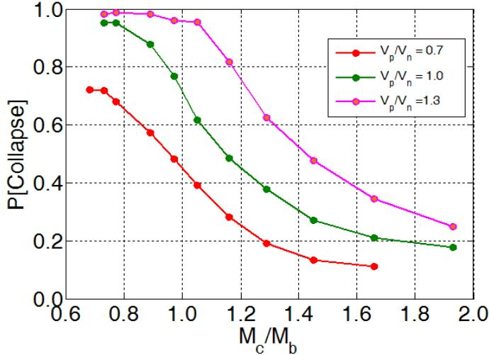
**Figure 10.** Probability of collapse at the MCE level for different  $V_p / V_n$  and  $\Sigma M_c / \Sigma M_b$  ratios
