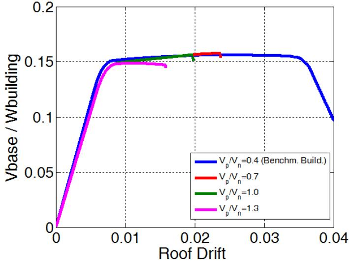
**Figure 7.** Pushover Analysis of model building for different  $V_p/V_n$  ratios
