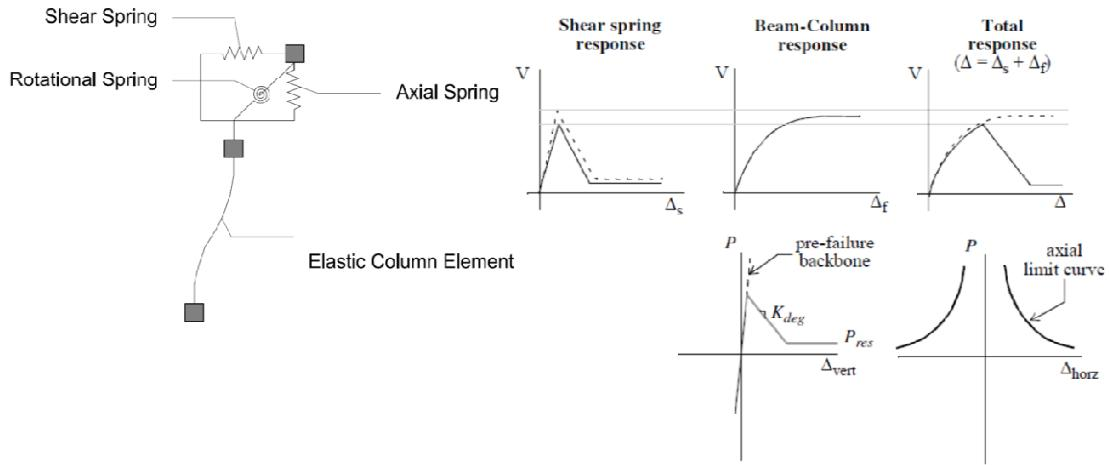
**Figure 6.** Limit State Material (developed by Elwood and Moehle)
