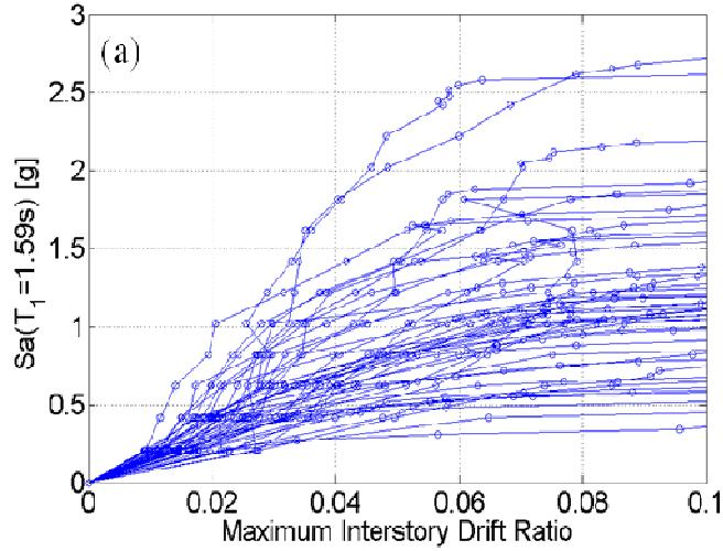
**Figure 8.** Incremental Dynamic Analysis (IDA) Results for “benchmark” building
