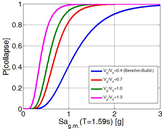
**Figure 9.** Fragility curves for different  $V_p/V_n$  ratios
