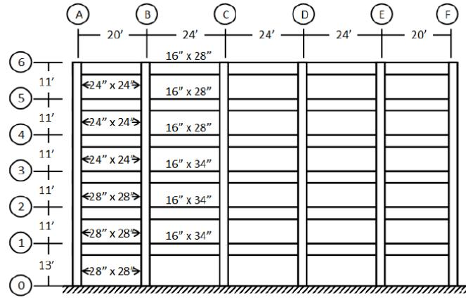
**Figure 2.** Elevation view of the perimeter frame
