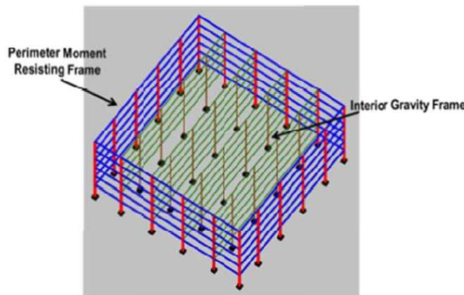
**Figure 1.** Three-dimensional view of the benchmark building
