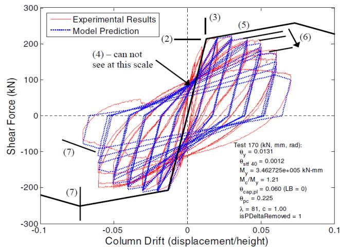
**Figure 4.** Response of a calibrated spring-column element (Haselton et al. PEER 2007/03)
