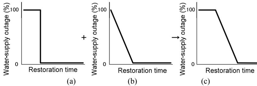
**Figure 4.** Schematic chart of water-supply restoration: (a) Facility, (b) Pipeline, and (c) Entire system
