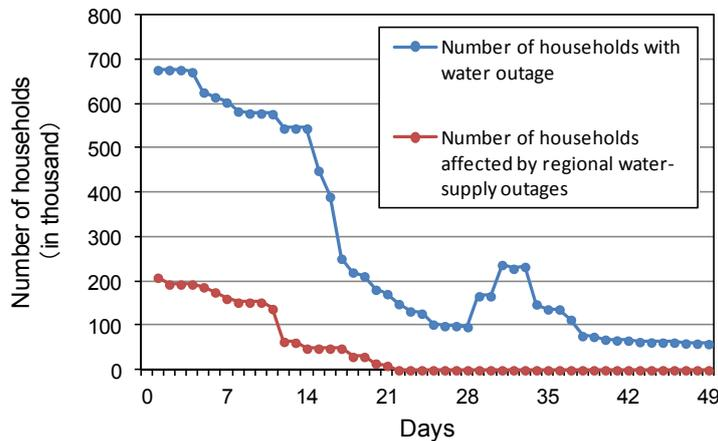
**Figure 8.** Number of households with water outage following the Tohoku earthquake in Miyagi Prefecture.
