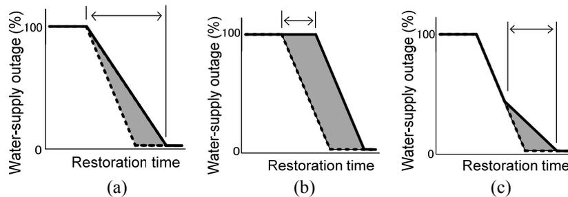
**Figure 5.** Concept of restoration time due to the following factors: (1) Delay in pipeline restoration, (2) Power-supply outage at the water facility and/or outage of the regional water-supply, (3) Delay due to pipeline repair in a liquefaction area
