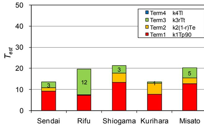
**Figure 9.** Estimated restoration times for the water supply with composition for restoration times due to regional water-supply outage
