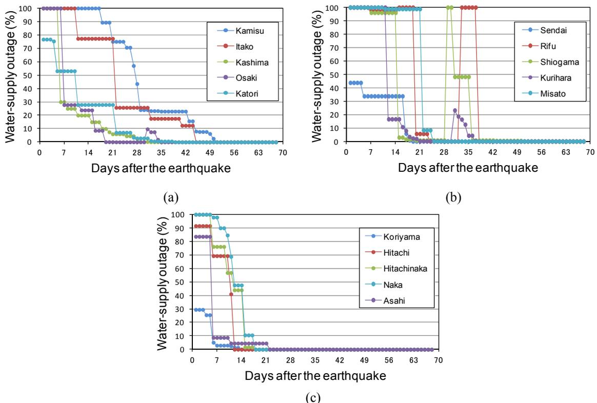
**Figure 3.** Restoration process of the water supply: (a) Water-supply authorities affected by the regional water-supply outage, (b) Water-supply authorities affected by large-area liquefaction, and (c) Water-supply authorities not affected by special factors.
