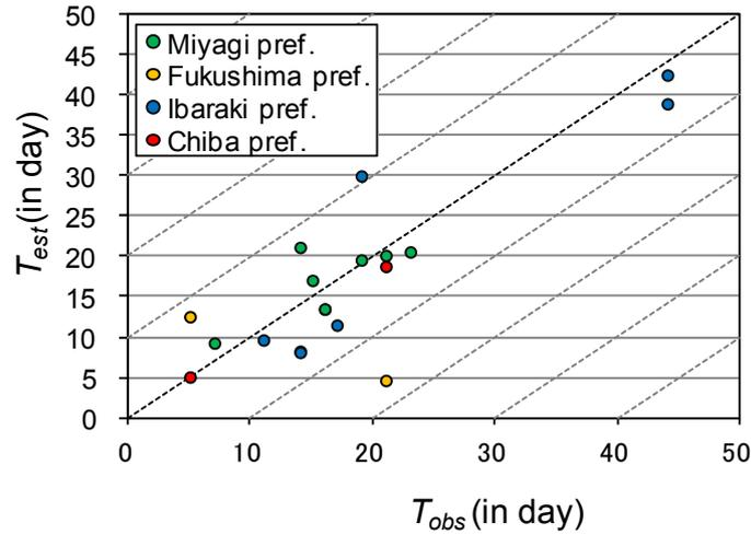
**Figure 7.** Relationship between actual 90% restoration time,  $T_{obs}$ , and the 90% restoration time estimated by the enhanced model,  $T_{est}$ , for 19 affected water-supply authorities
