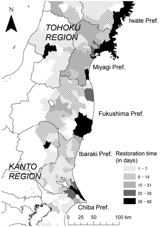
**Figure 1.** Restoration time for water-supply system in water-supply districts following the Tohoku earthquake
