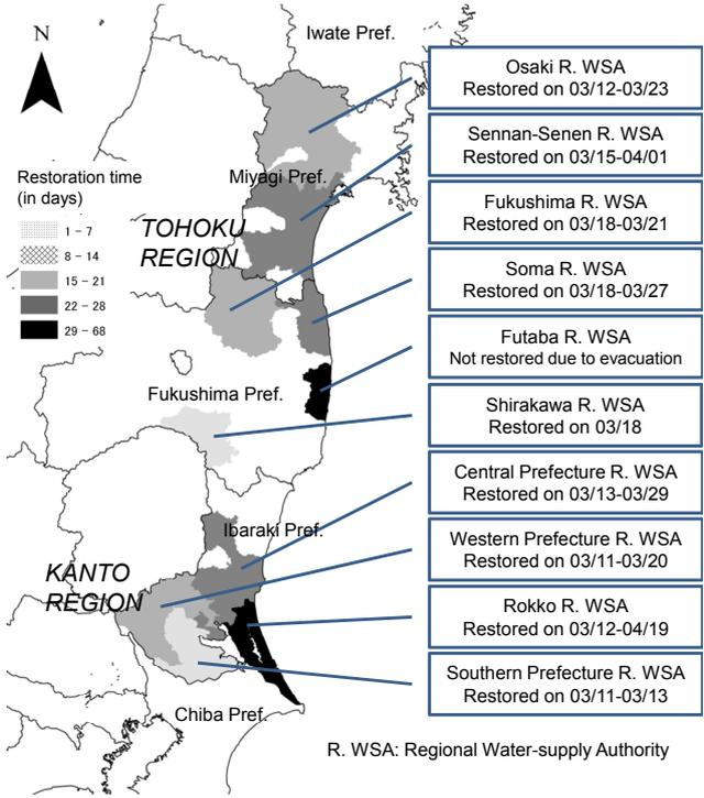
**Figure 2.** Restoration time for the regional water-supply systems following the Tohoku earthquake
