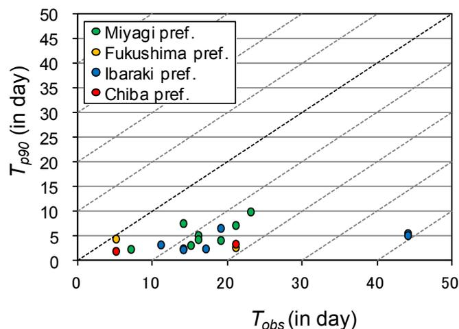
**Figure 6.** Relationship between actual 90% restoration time,  $T_{obs}$ , and the 90% restoration time estimated by the pipe repair rate,  $T_{p90}$ , for 19 affected water-supply authorities
