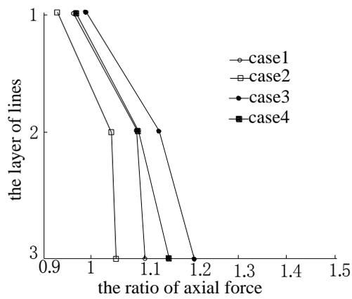
**Figure 4.4.** The ratio of axial force to the lines
