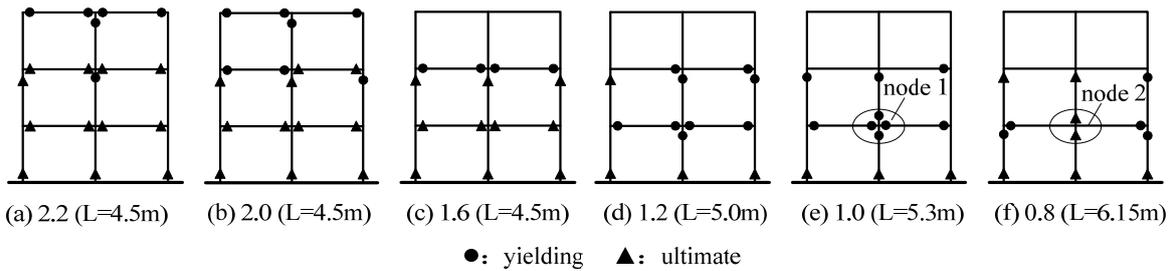
**Figure 4.4.** Comparison of ultimate failure modes for different  $\beta_c$
