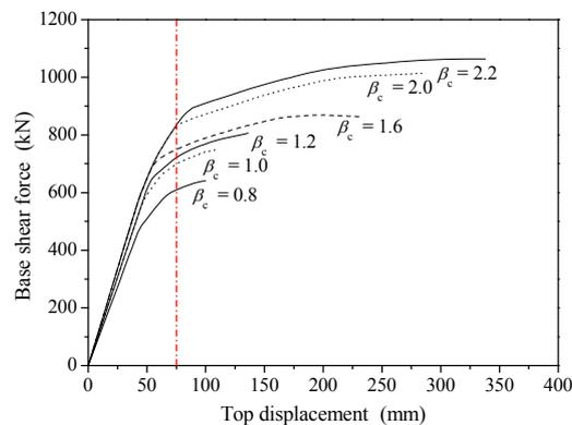
**Figure 4.1.** Comparisons of capacity curves for different  $\beta_c$
