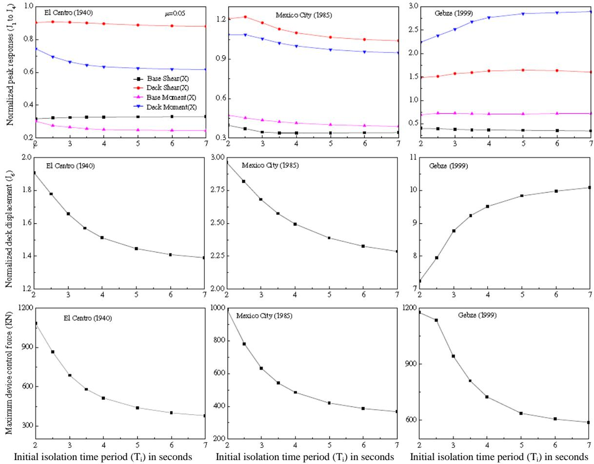
**Figure 4. Effect of initial time period of VCFPS on normalized responses of the bridge**
