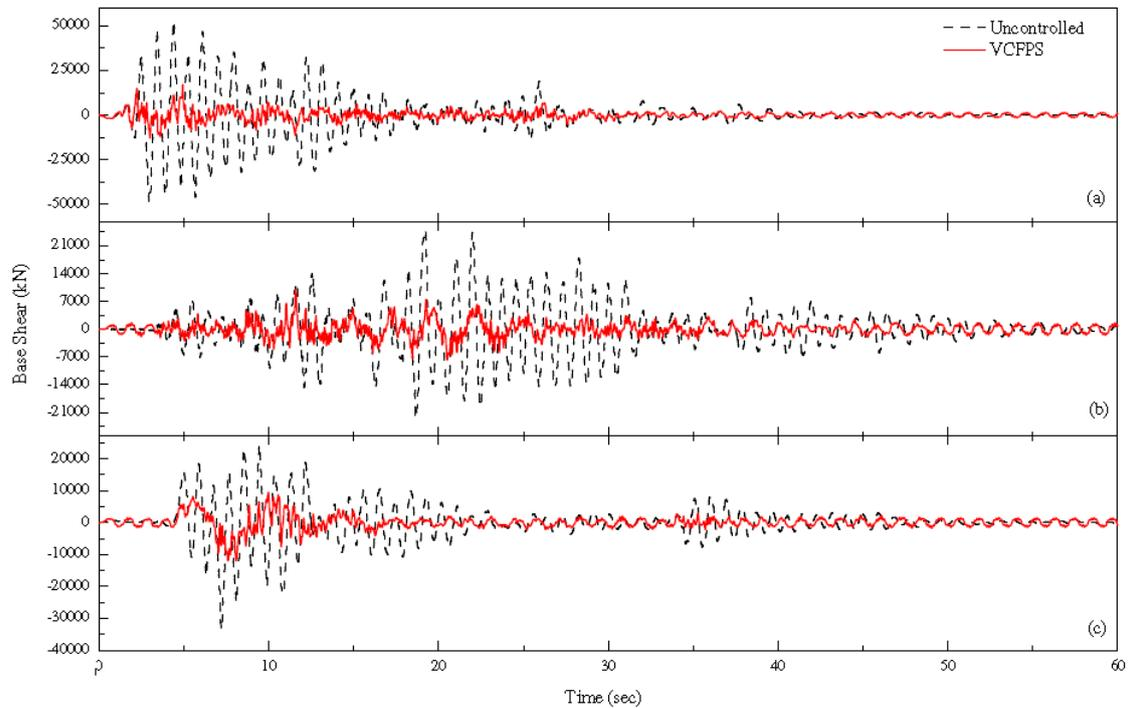
**Fig. 6 Uncontrolled and VCFPS controlled Base Shear response for (a) El Centro (1940), (b) Mexico City (1985) and (c) Gebze (1999) earthquakes at pier 2**
