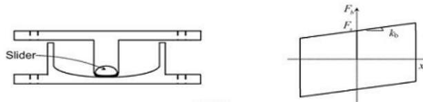
**Figure 2. Friction Pendulum System (FPS)**
