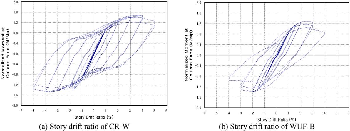
Figure 11. Hysteretic curves of story drift ratio
