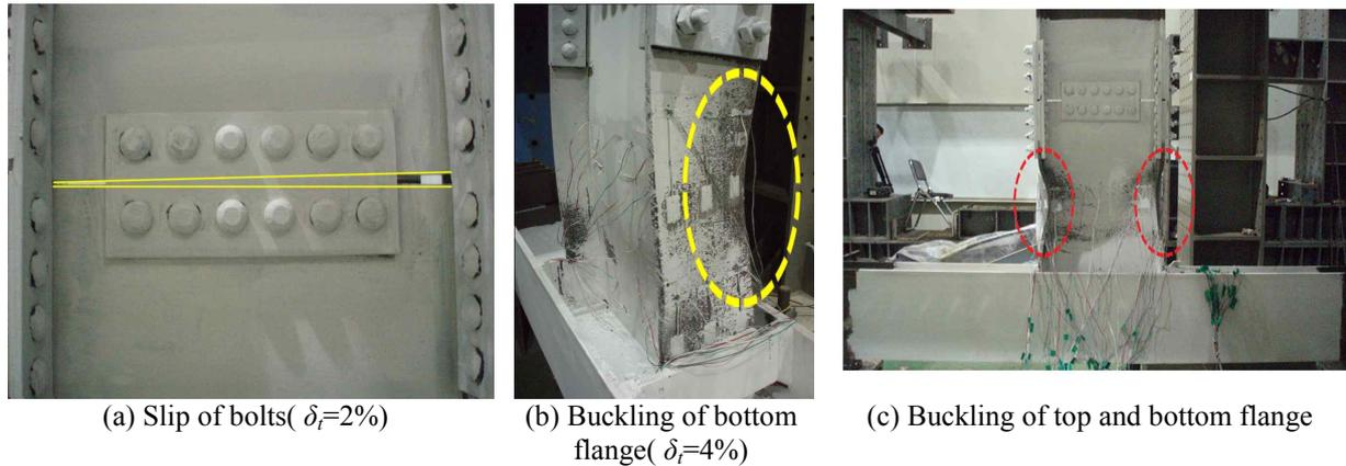
**Figure 9.** Failure shapes of CT-W specimen
