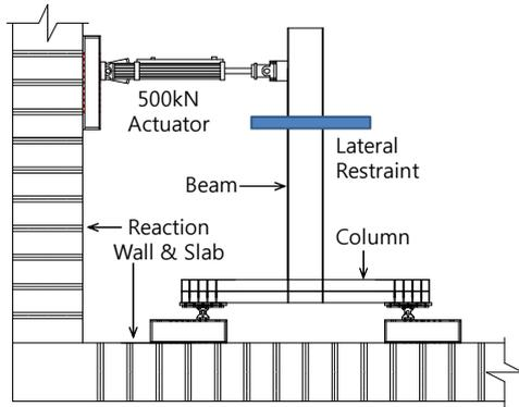
Figure 5. Test setup
