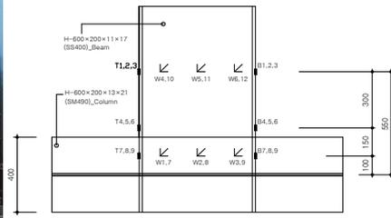
Figure 6. Gauges Layout
