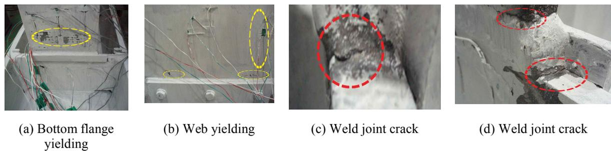
**Figure 10.** Failure shapes of WUF-B specimen
