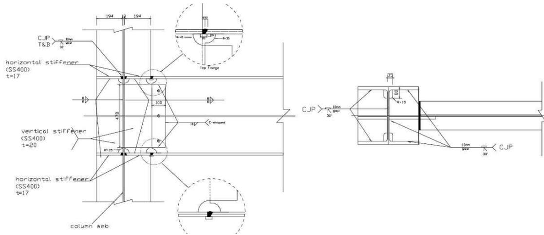
Figure 3. WUF-B type specimen
