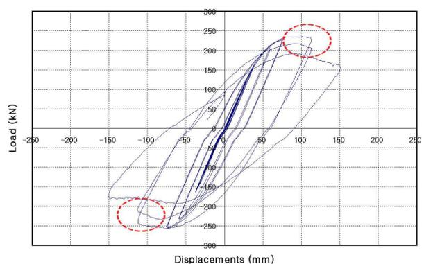
Figure 8. Load-displacement Curve for WUF-B
