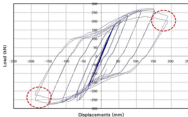
Figure 7. Load-displacement Curve for CT-W
