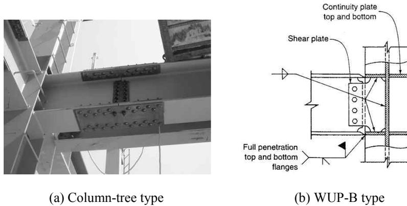
**Figure 1.** The details of weak-axis connections
