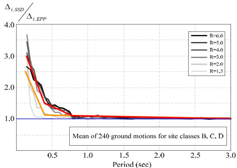
**Figure 3.** Mean displacement ratio of SSD to EPP models ( $C_2$ ) computed with ground motions recorded on site classes B, C, and D. (FEMA 440, 2006)
