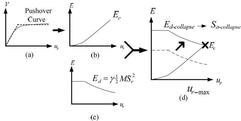
**Figure 5.** Proposed energy-based evaluation method for MDOF systems: (a) Push-over curve, (b) Energy-displacement capacity diagram, (c) Energy demand diagram, and (d) Determination of  $S_{a\text{-collapse}}$
