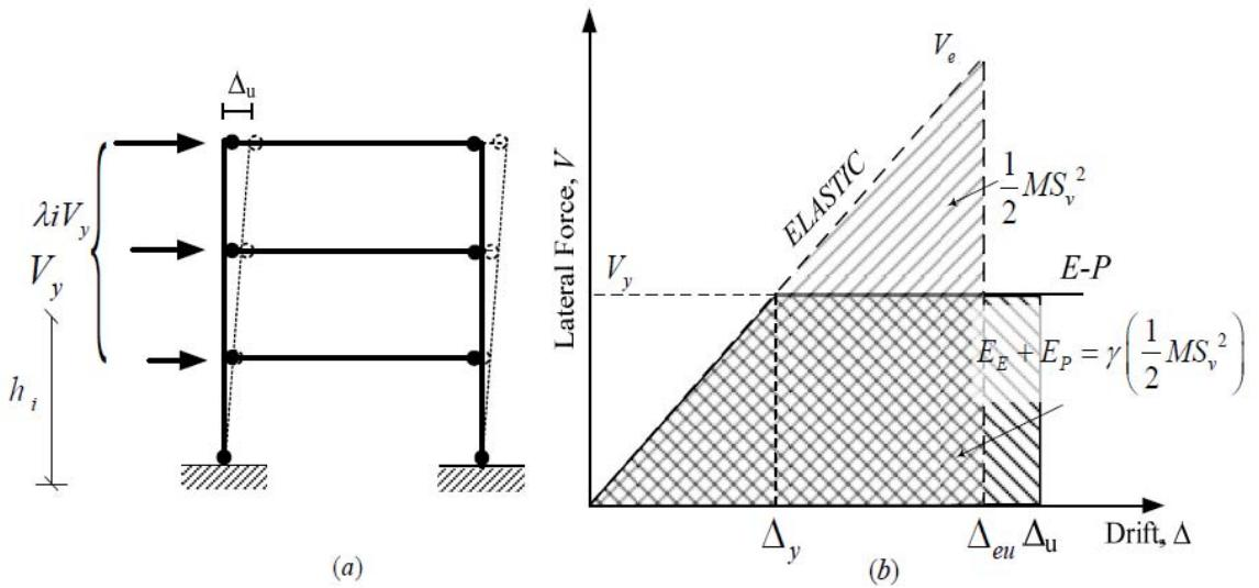
**Figure 2.** Energy balance concept in PBPD (Lee and Goel, 2001).
