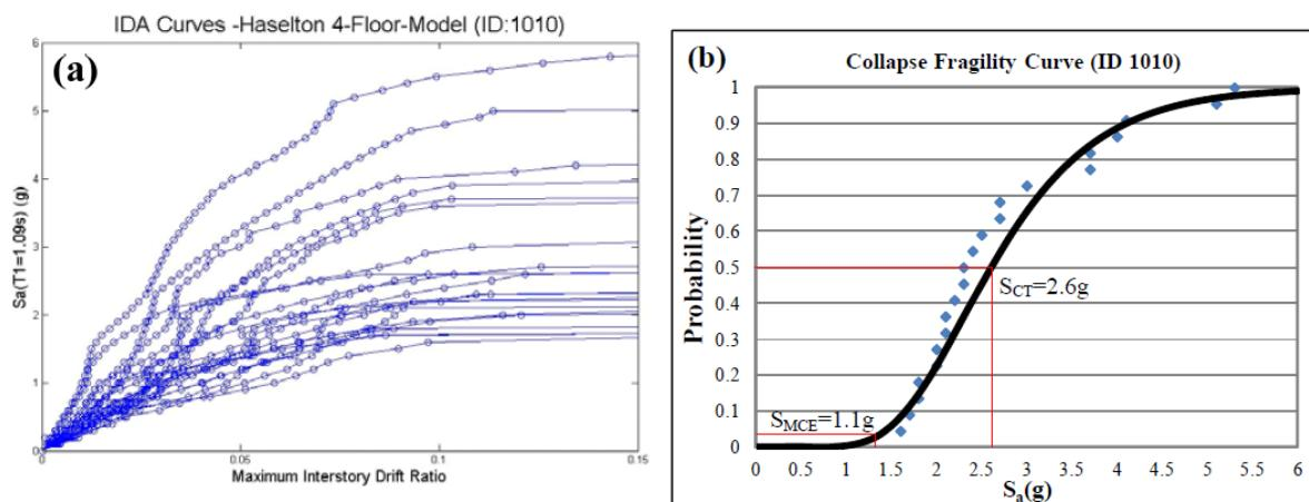
**Figure 1.** Incremental dynamic analysis (a) IDA plot of  $S_a$  versus maximum interstory drift, (b) collapse fragility curve
