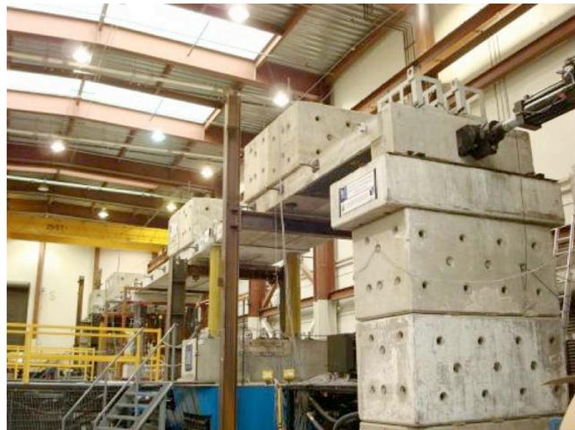
Figure 3. The Bridge Model with Glass Fiber Reinforced Polymer Wrapped Columns mounted on three shake tables at the University of Nevada, Reno (UNR) NEES Laboratory
