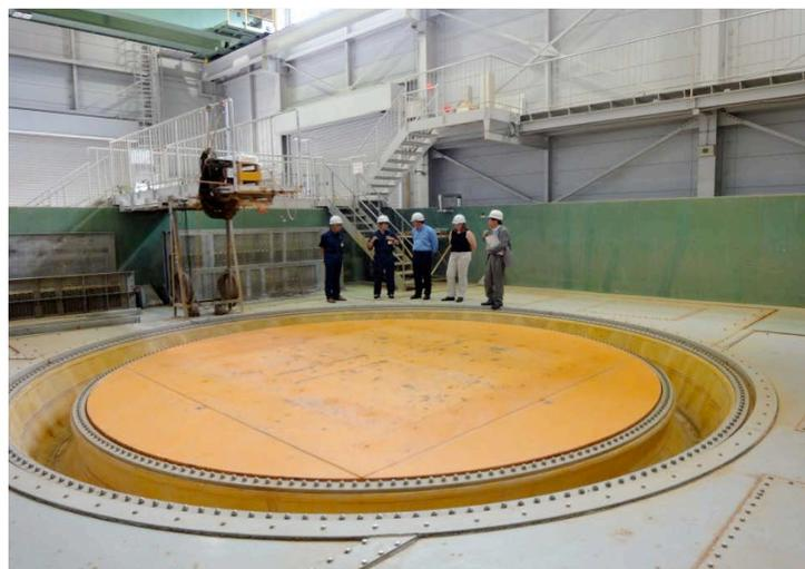
Figure 9. PARI Underwater Shake Table (UST)
