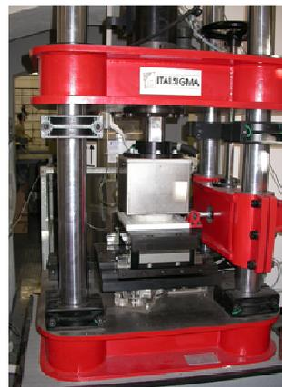
**Figure 3.1:** Bearing Tester System (left) and Sliding Material Tester (right).
