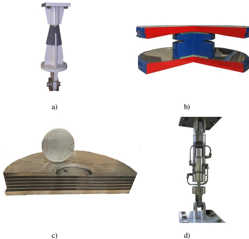
**Figure 1.1:** Examples of anti-seismic devices: a) hysteretic steel device (Displacement Dependent Device); b) sliding pendulum (Curved Surface Sliding Isolator); c) high damping rubber bearing (Elastomeric Isolator); d) Fluid Viscous Damper (Velocity Dependent Device)
