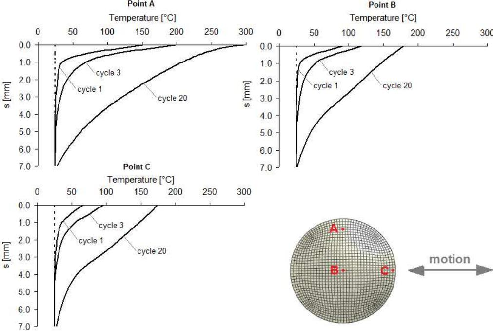
**Figure 4.7.** Temperature profiles through the thickness of the sliding pad during 20 cycles of motion in correspondence of positions marked as A, B, C
