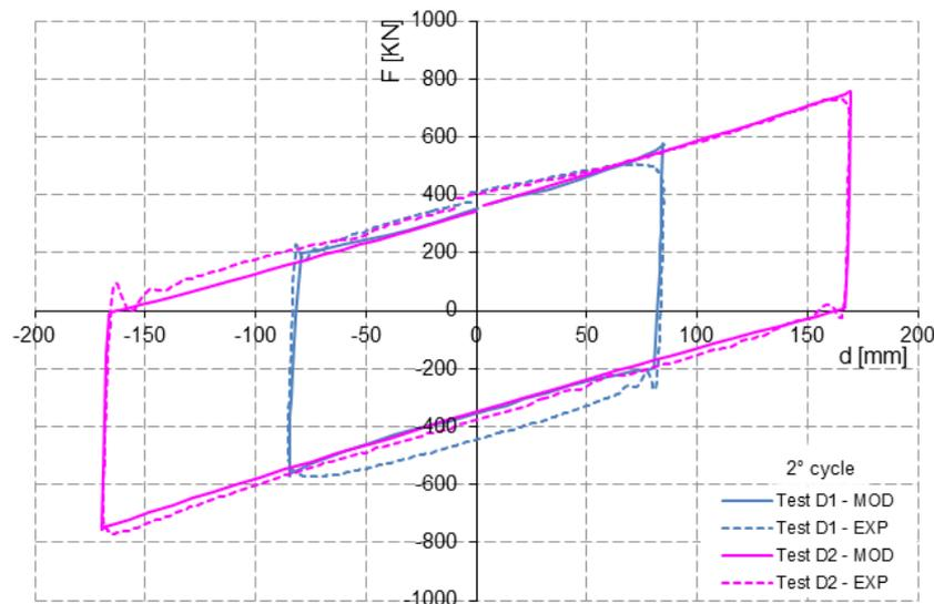
**Figure 2.2.** Hysteretic load – displacement diagrams of the CSS unit during cycles of horizontal loading at displacement amplitude  $d = 85$  mm (D1) and  $d = 170$  mm (D2) and period  $T = 2.13$  s: comparison between finite element simulations (MOD) and experimental data (EXP)
