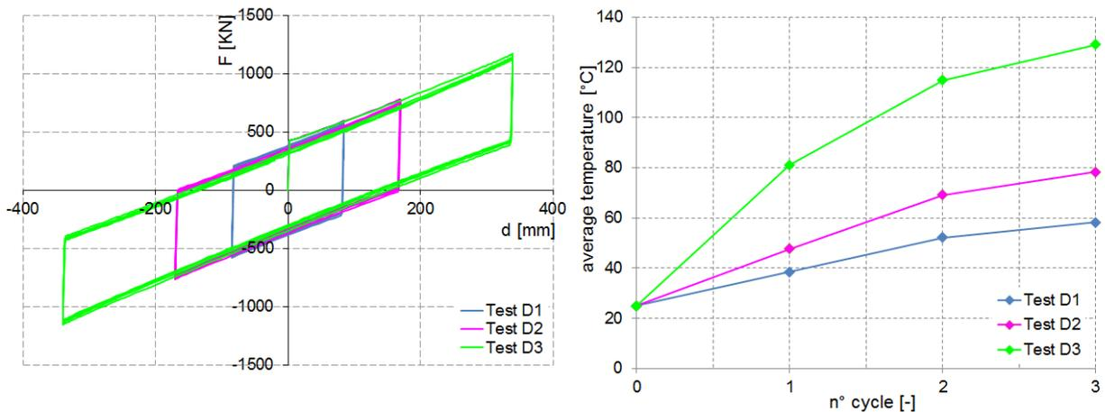
**Figure 4.1.** Load – displacement diagrams and cycle histories of average temperature on the surface of the sliding pad of the CSS unit during test D1, D2 and D3
