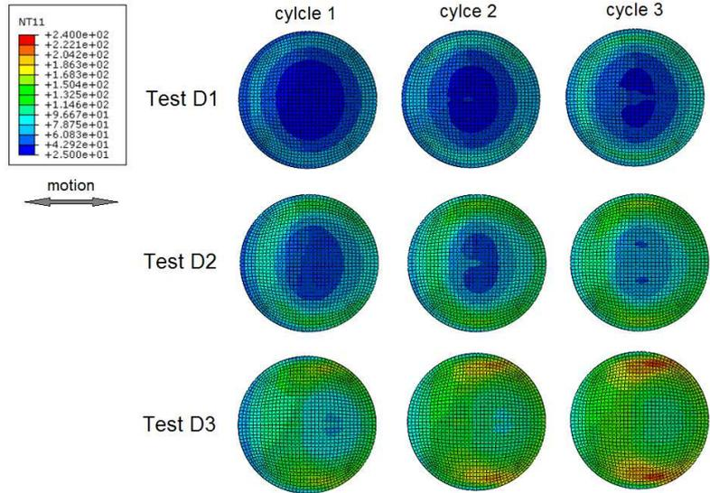
**Figure 4.3.** Temperature profiles on the surface of the sliding pad during Tests D1, D2 and D3 (values in °C)
