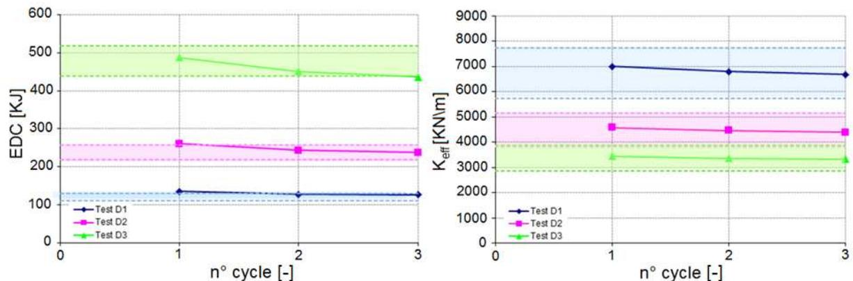
**Figure 4.2.** Change of Energy Dissipated per Cycle ( $EDC$ ) and Effective Stiffness ( $K_{eff}$ ) during repeated cycles at different speeds and range of acceptability (colored strips) according to EN 15129
