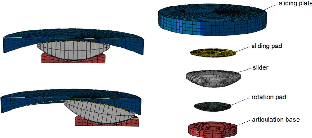
**Figure 2.1.** Finite element mesh of the CSS unit: typical operation (left) and details of its component parts (right)
