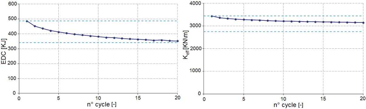
**Figure 4.6.** Change of Energy Dissipated per Cycle ( $EDC$ ) and effective stiffness ( $K_{eff}$ ) during repeated cycles and range of acceptability according to AASHTO
