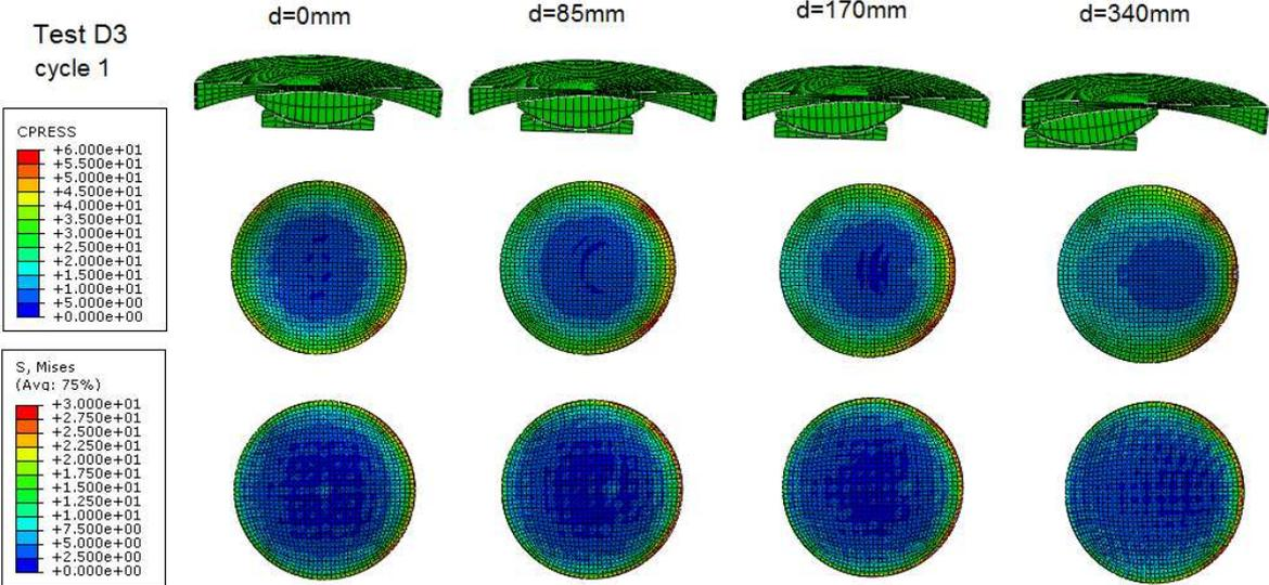
**Figure 4.4.** Distribution of contact (CPRESS) and Von Mises (S. Mises) stresses on the surface of the polymeric pad during the first cycle of Test D3 (values in MPa)
