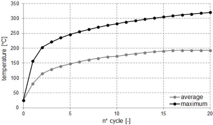
**Figure 4.5.** Average and maximum temperature histories on the surface of the sliding pad during Test D4 according to AASHTO
