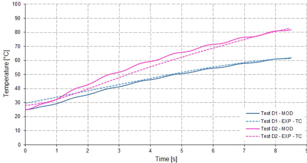
**Figure 2.3.** Peak temperature on the back of the stainless steel sliding surface during horizontal loading at displacement amplitude  $d = 85$  mm (D1) and  $d = 170$  mm (D2): comparison between finite element simulations (MOD) and thermocouple measurements (EXP)
