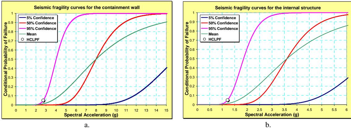
**Figure 4.** Seismic fragility curves for the containment wall and the internal structure.
