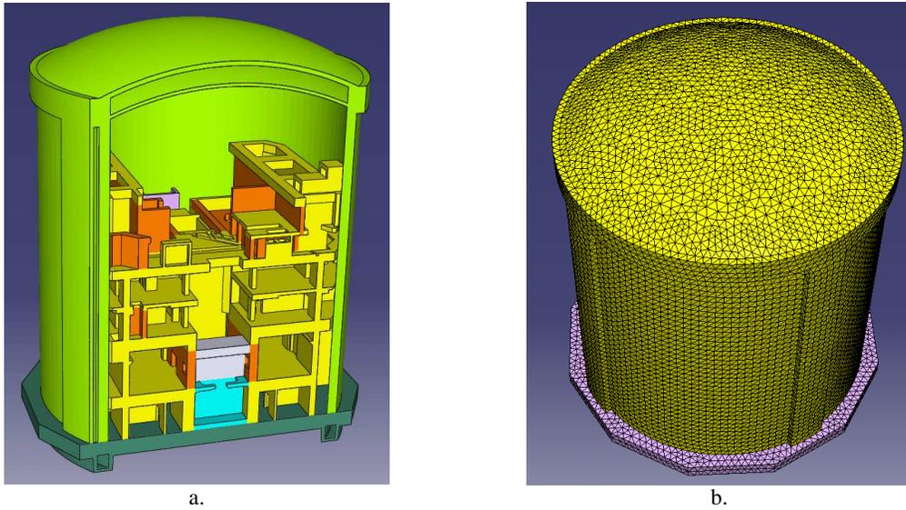
**Figure 2.** Finite element model of the CANDU 6 reactor building.
