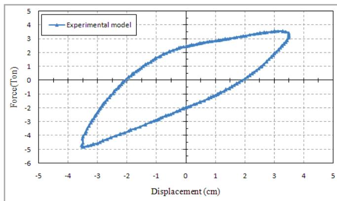
Figure 2.4. Last Hysteretic Loops of Two Layer Specimen
