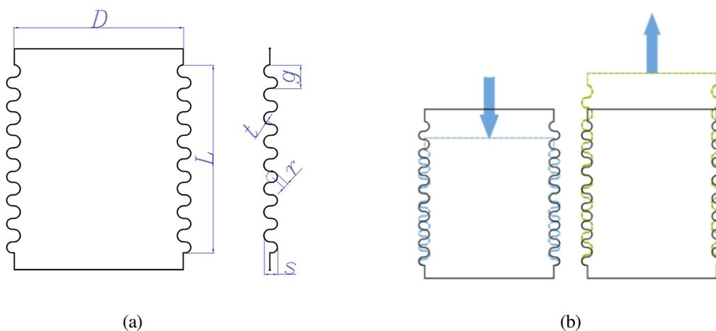
**Figure 2.1.** Schematic Overview of Specimens: Geometric Characteristics (a), Acting Load and Deformation (b)
