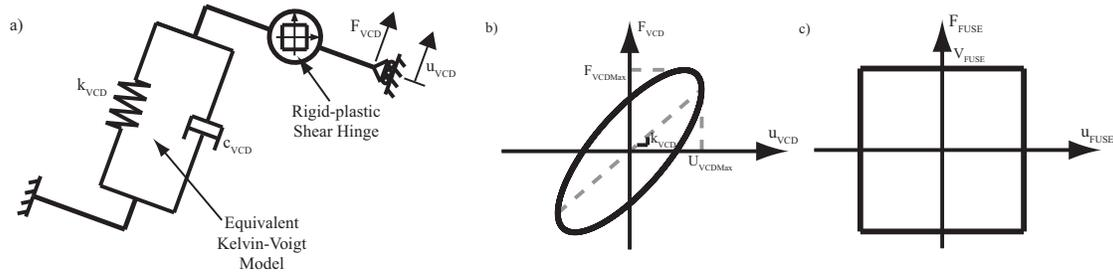
**Figure 5.1** a) Schematic of VCD model, b) Viscoelastic VCD hysteresis, c) Rigid-plastic shear hinge hysteresis
