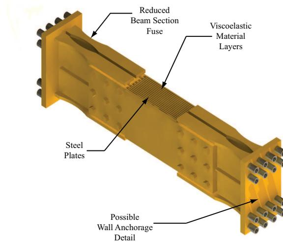
**Figure 2.1** Viscoelastic Coupling Damper (VCD)
