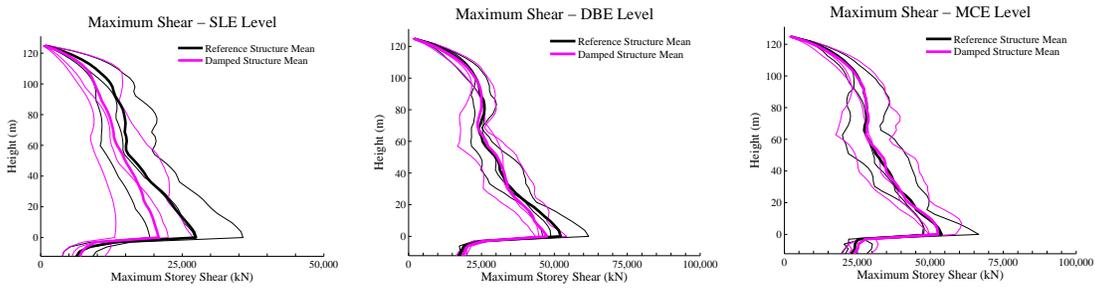
**Figure 9.4** Maximum Storey Shear – North-South Direction
