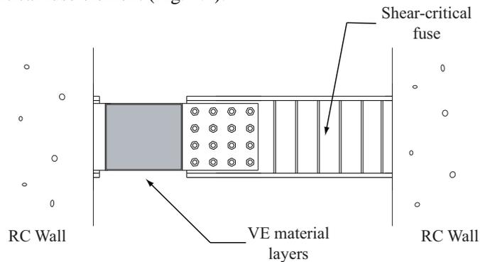
**Figure 4.1** Shear force limiting VCD
