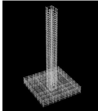
**Figure 3.1** Perform-3D model of prototype building
