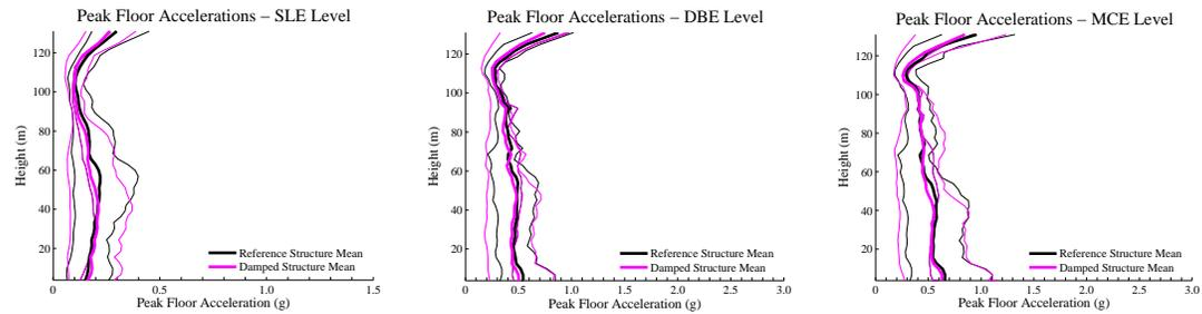
**Figure 9.5** Maximum Storey Acceleration – East-West Direction
