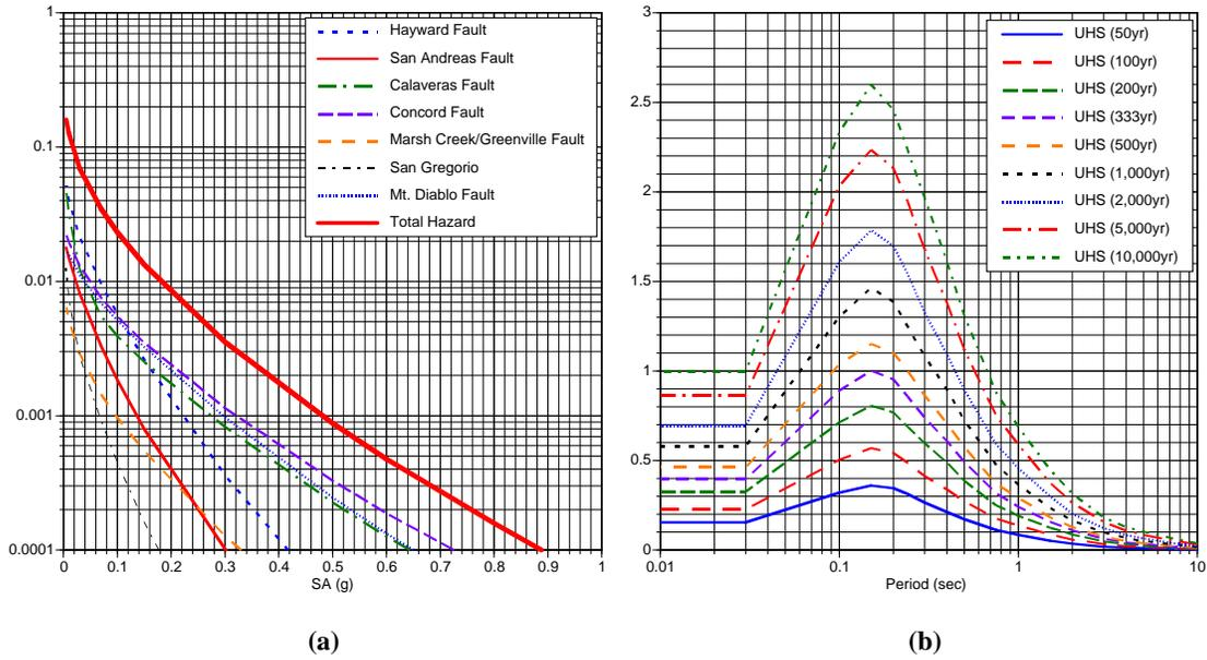
**Figure 1.** (a) Hazard curve for contributing faults at  $T=0.75$  sec., plotted as spectral acceleration versus probability of exceedance in one year. (b) Spectra for various hazard levels, plotted as period versus  $S_a$ .
