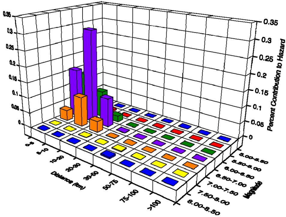
**Figure 2.** Hazard de-aggregation for  $T=0.75$  sec. spectral period at the 2,000 year return period.
