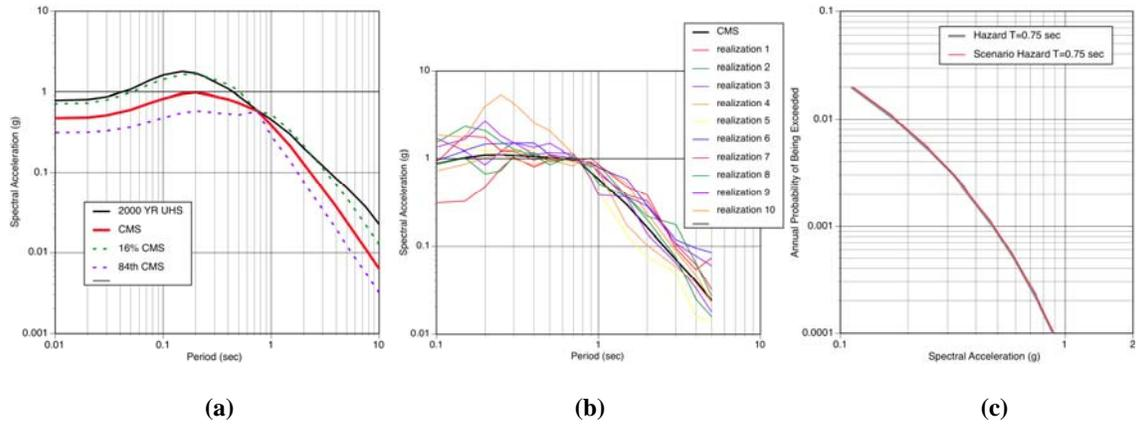
**Figure 3.** (a) CMS constructed from the hazard de-aggregation for  $T=0.75$  sec. and a 2,000 year return period. (b) Scenario spectra constructed for one of the CMS. (c) Hazard curve recreated from the 120 scenarios as a check for  $T=0.75$  sec.
