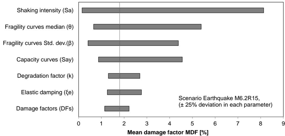
**Figure 5.1.** Variation of the predicted MDF for different input parameters in vulnerability analysis for stone masonry buildings.
