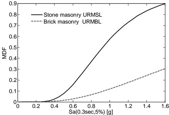
**Figure 3.4.** Seismic vulnerability functions for stone and brick masonry buildings.
