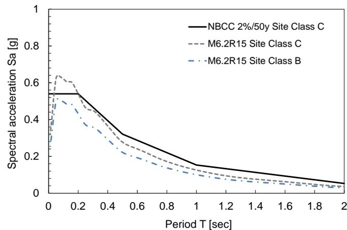
**Figure 3.2.** Response spectra for the selected M6.2R15 scenario on site class C (very dense soil and soft rock) and B (rock), and the NBCC 2%/50 years uniform hazard spectrum for Quebec City for site-class C.
