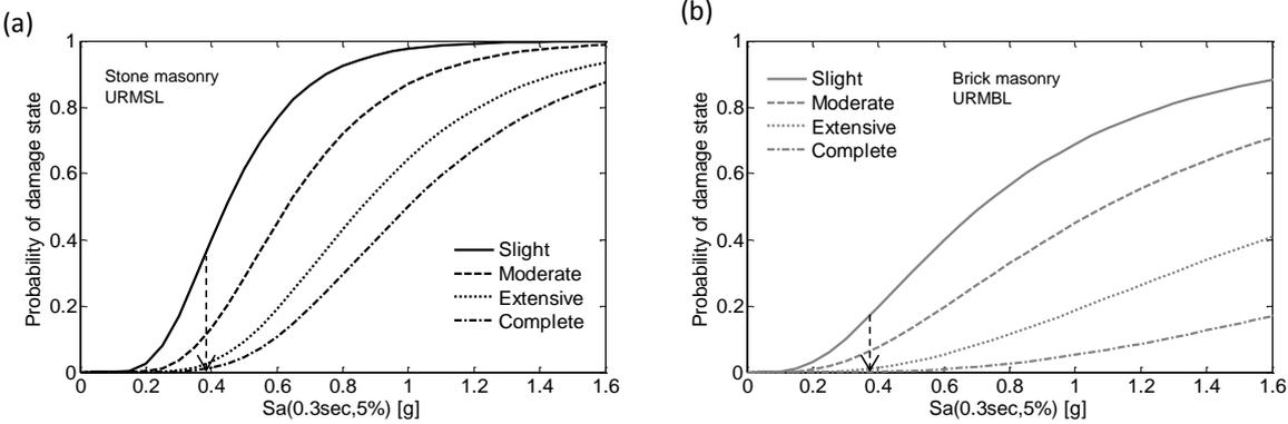
**Figure 3.3.** Fragility functions for (a) stone masonry buildings, and (b) brick masonry buildings. The dotted arrow shows the IM for the selected scenario M6.2R15.
