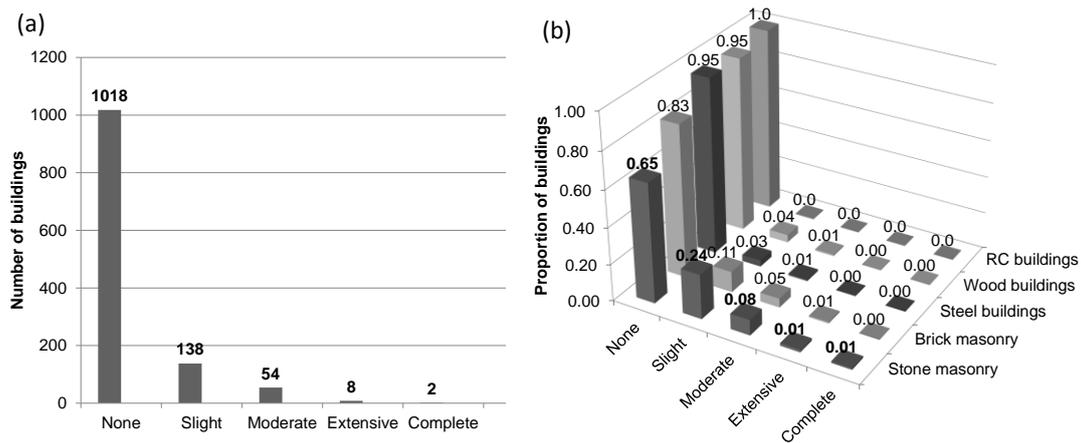
**Figure 4.1.** a) Total number of buildings in each damage state, b) proportion of buildings by construction material type in each damage state for a scenario event M6.2R15.
