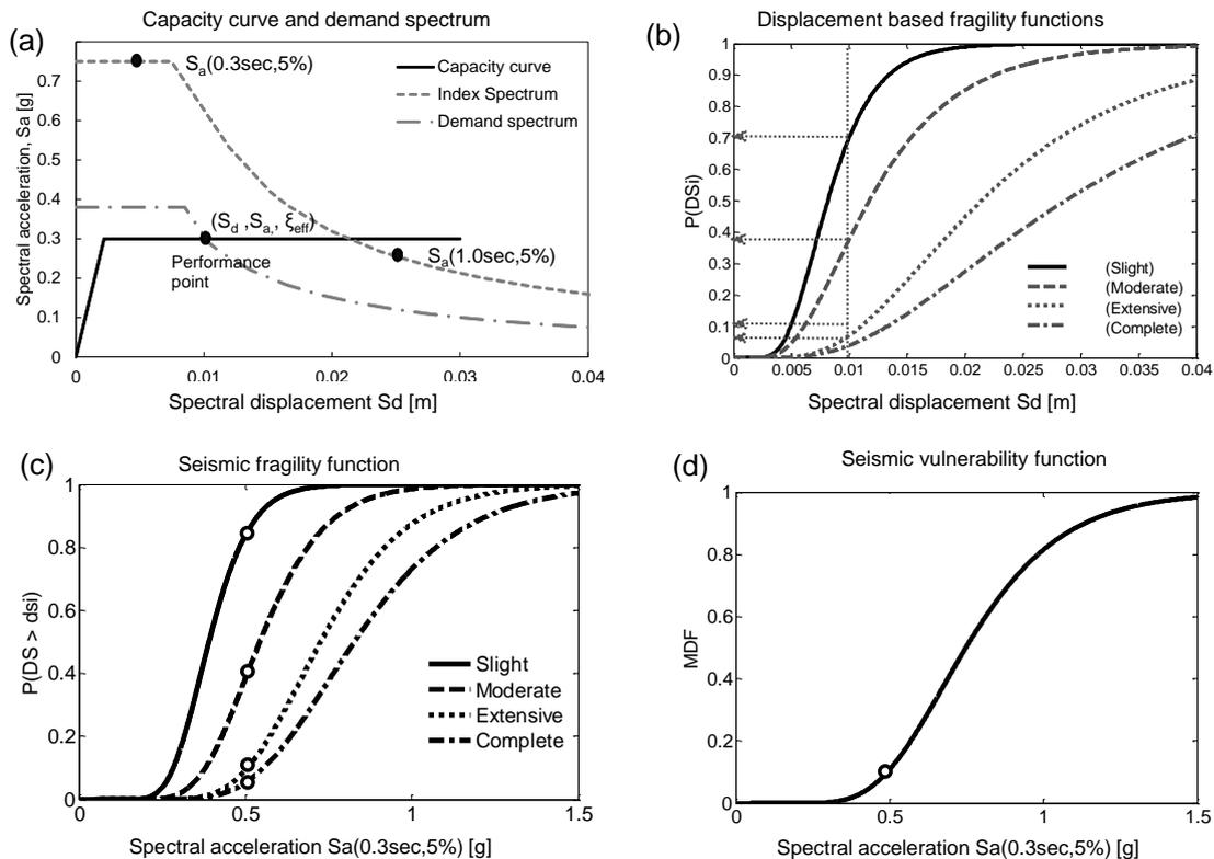
**Figure 2.1.** Illustration of the vulnerability modelling procedure (a) definition of the performance point; (b) estimation of the probability of damage states; (c) conversion of the fragility functions against spectral acceleration; (d) development of the vulnerability function in terms of MDF.
